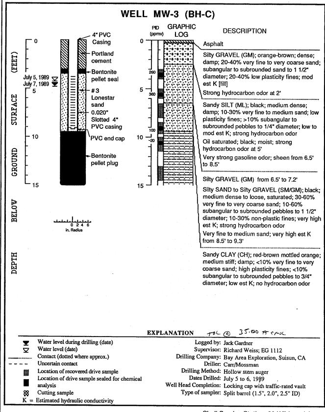
Well Construction and Boring Log - Well MW-3 (BH-C)
