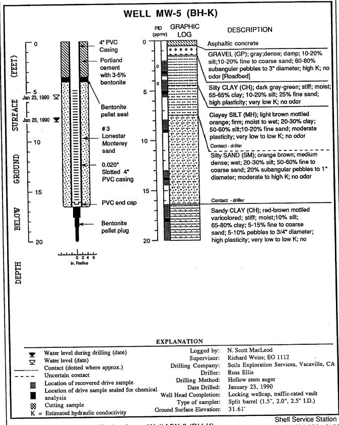
Well Construction and Boring Log - Well MW-5 (BH-K)
