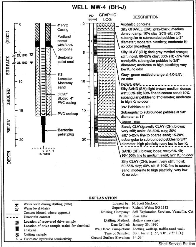
Well Construction and Boring Log - Well MW-4 (BH-J)
