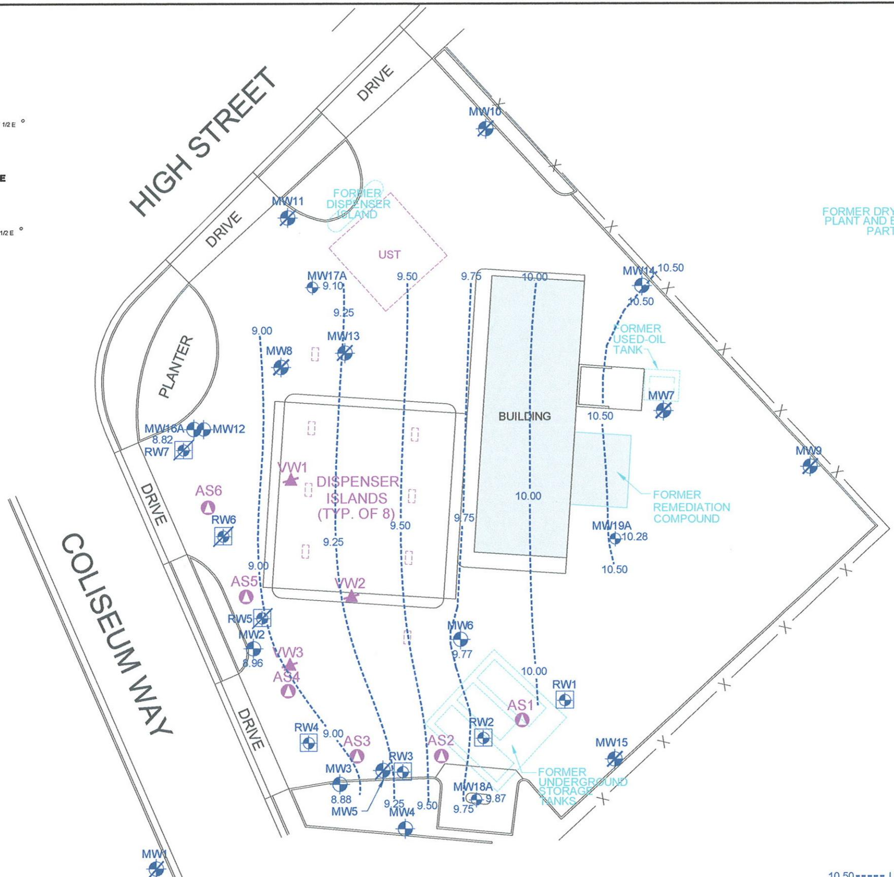
10.50 ----- Line of Equal Groundwater elevation;
