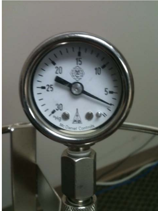
Plate 9. Pressure gauge on air sample canister post sampling
