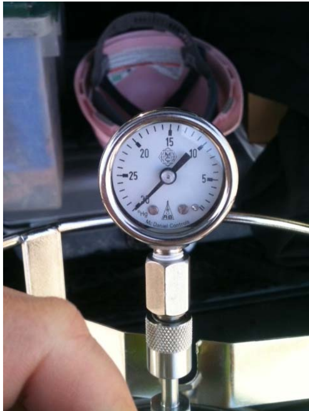
Plate 8. Pressure gauge on air sample canister prior to sampling
