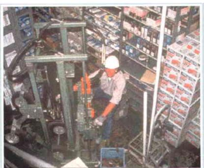
**DA Series** (Hand-truck) This the rig to use when the access is very limited. As you see in this photo getting into small spaces is no problem for this rig. The power unit is connected to the rig by a long hydraulic hose. Fits through commercial doorways. Capable of angle borings to 35 degrees. Although small in size, these rigs can core soil to 50 feet.
