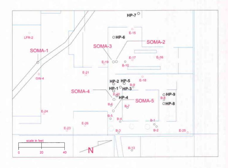
Figure 1: Location of New Installed Groundwater Monitoring Wells
