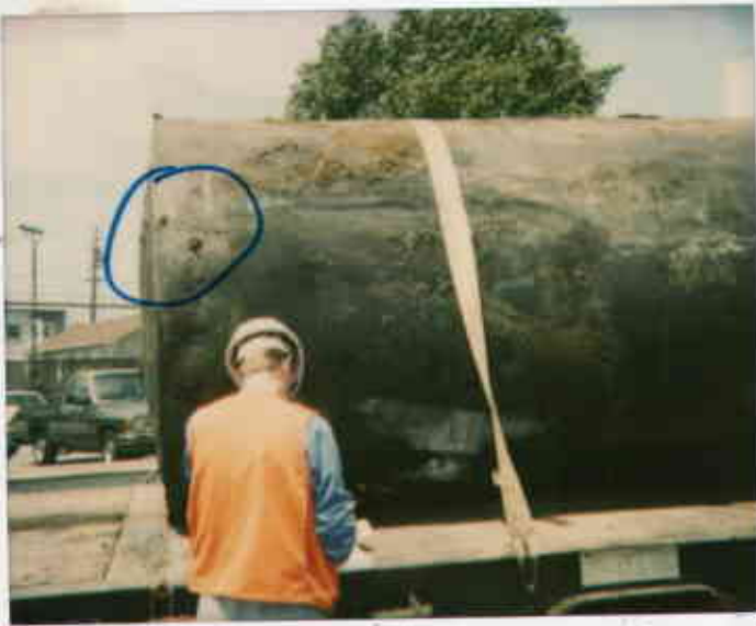
Tank B (w/ hole on the side) 5/18/94 ST10567
