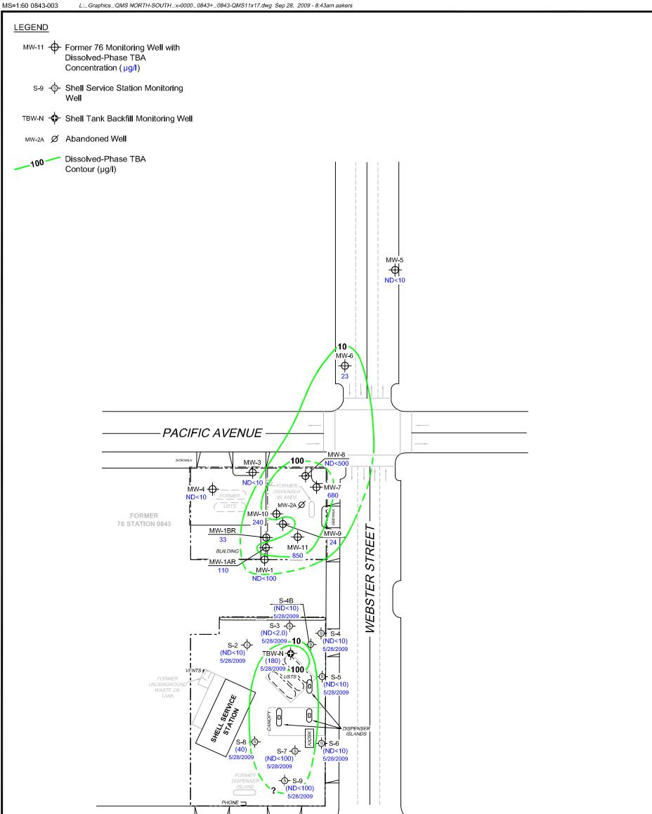
Contour lines are interpretive and based on laboratory analysis results of groundwater samples. TBA = tertiary butyl alcohol. μg/l = micrograms per liter. ND = not detected at limit indicated on official laboratory report. Dashes indicate contour based on non-detect at elevated detection limit. ( ) = representative historical value. UST = underground storage tank. Shell Service Station data not provided this quarter. Results obtained using EPA Method 8260B.
