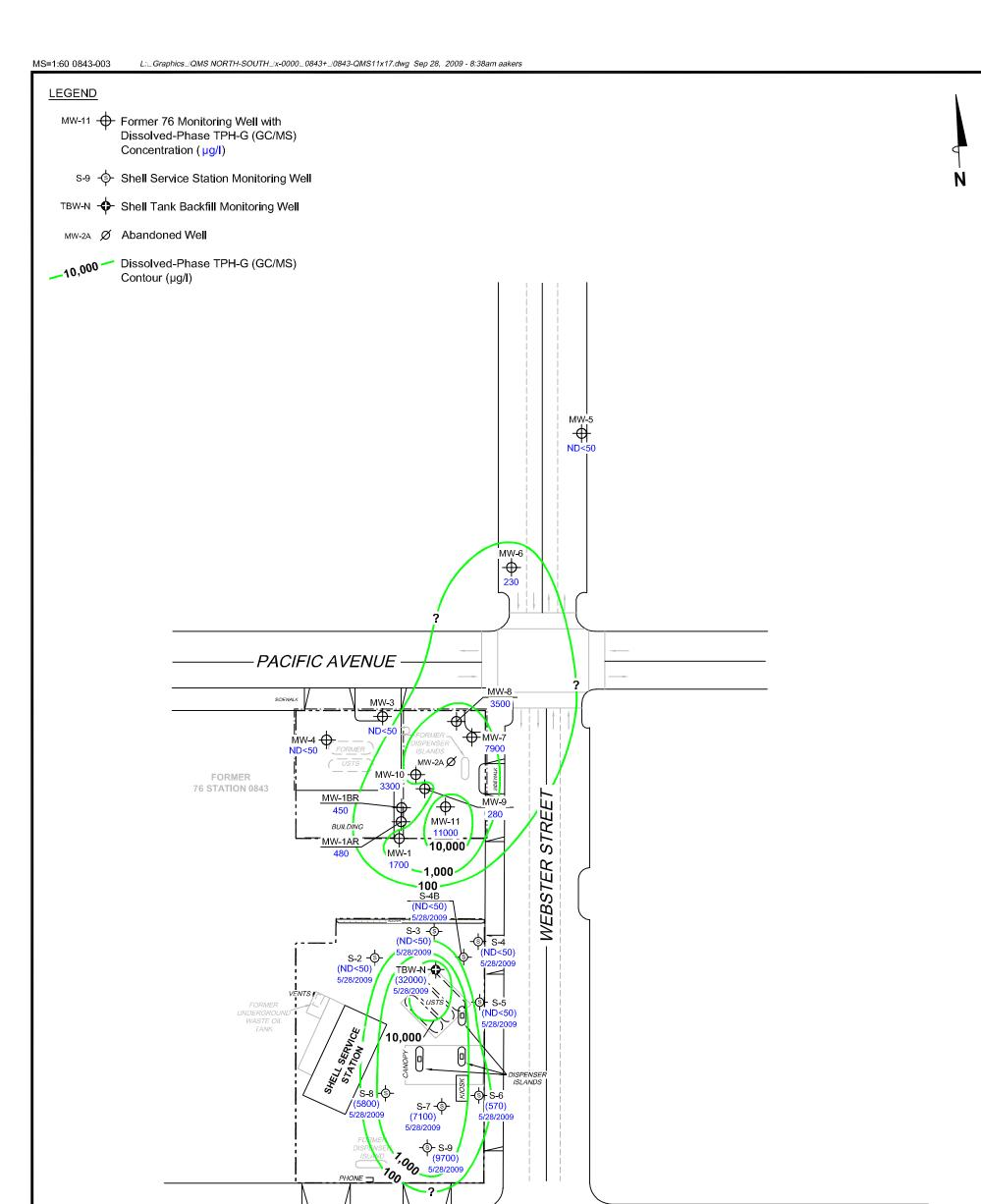
Contour lines are interpretive and based on laboratory analysis results of groundwater samples. TPH-G (GC/MS) = total petroleum hydrocarbons with gasoline distinction utilizing EPA Method 8260B.  $\mu$ g/l = micrograms per liter. ND = not detected at limit indicated on official laboratory report. ( ) = representative historical value. UST = underground storage tank. Shell Service Station data not provided this quarter.
