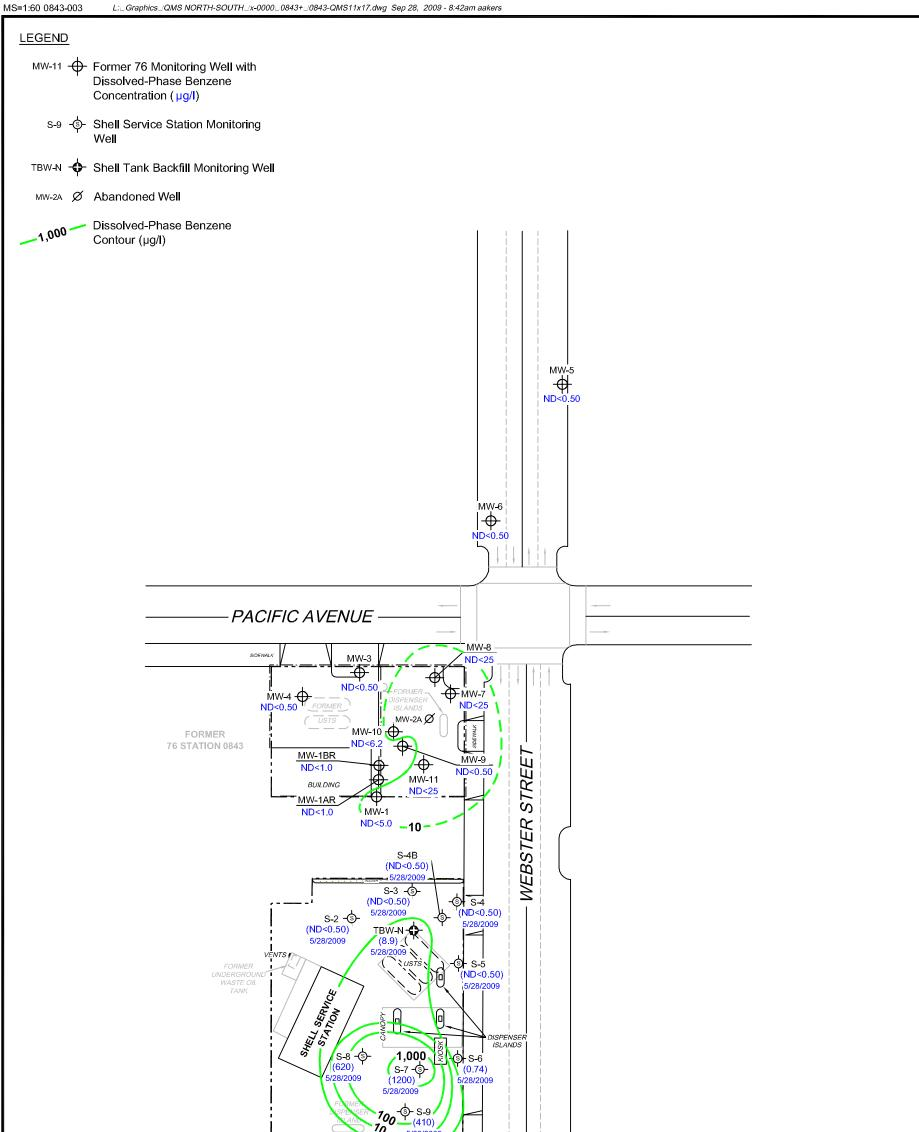
Contour lines are interpretive and based on laboratory analysis results of groundwater samples.  $\mu$ g/I = micrograms per liter. ND = not detected at limit indicated on official laboratory report. Dashes indicate contour based on non-detect at elevated detection limit. ( ) = representative historical value.  ${\sf UST = underground\ storage\ tank.\ \ Shell\ Service\ Station\ data\ not\ provided\ this\ quarter.}$
