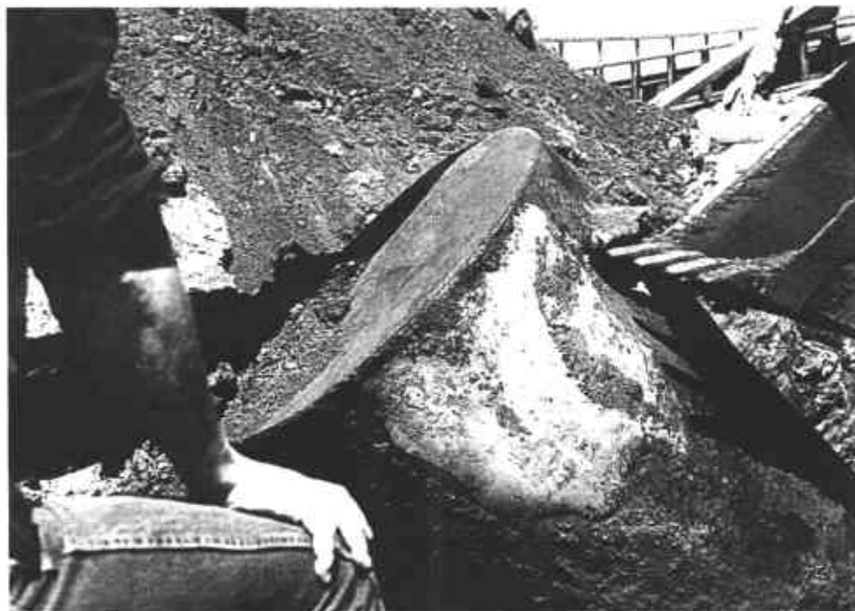
PHOTO 4: Close-up of rupture created during removal.
