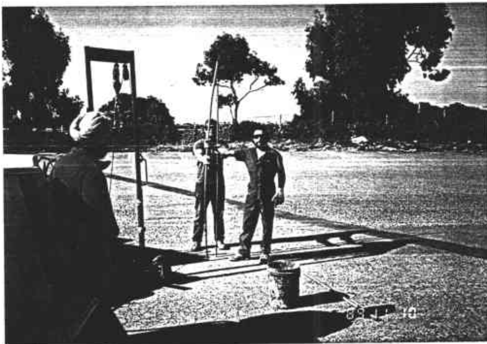
BENT SAMPLING PROBE FROM DRILL REFUSAL NEAR GROUNDWATER "GRAB" SAMPLE LOCATION GW-4
