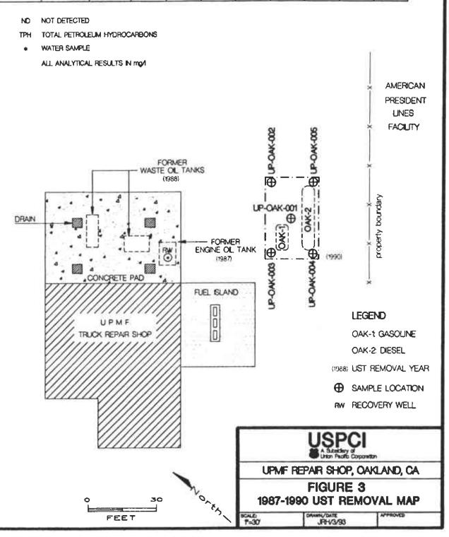
from the PSA indicated that there are detectable concentrations of contaminants in both soil and groundwater beneath the site. The findings suggested that the USTs are the likely source of petroleum hydrocarbons that were found in the groundwater, but not necessarily the source of the soil contamination.
