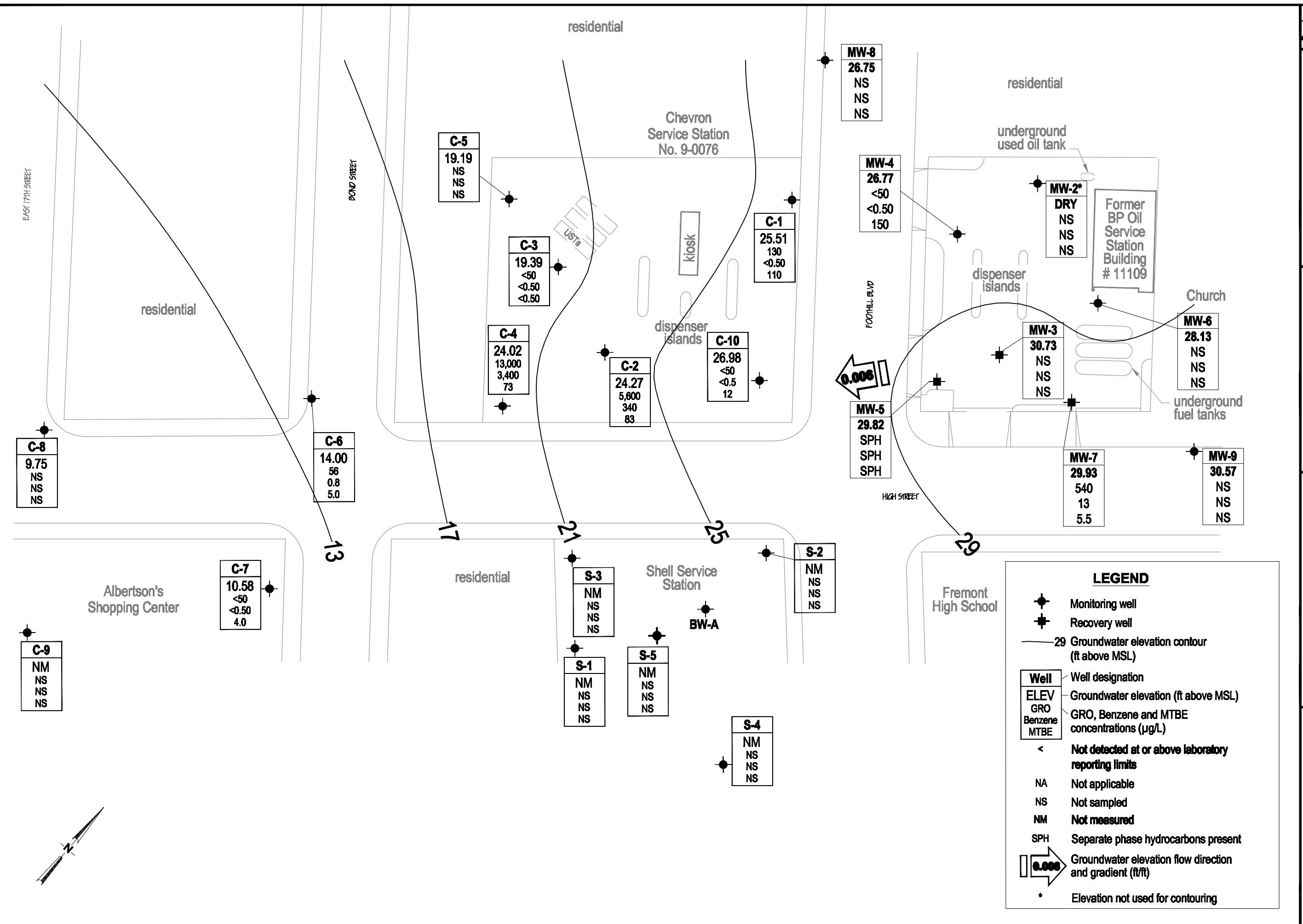
Table 1. Summary of Ground-Water Monitoring Data: Relative Water Elevations and Laboratory Analyses
