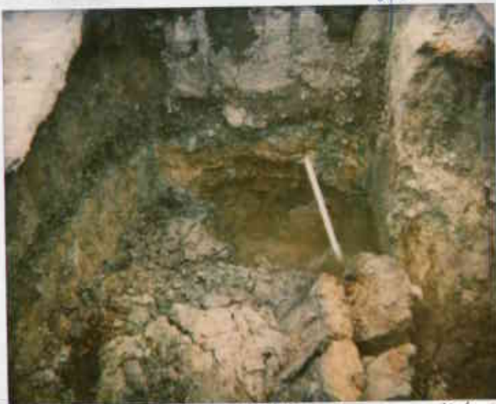
3530 MacArthur, Oakland 5/24/99 12215117976-B Sampled g.w. after pumping yesterday afternoon & letting it recharge. Slight sheen on water. Juliet Shui
