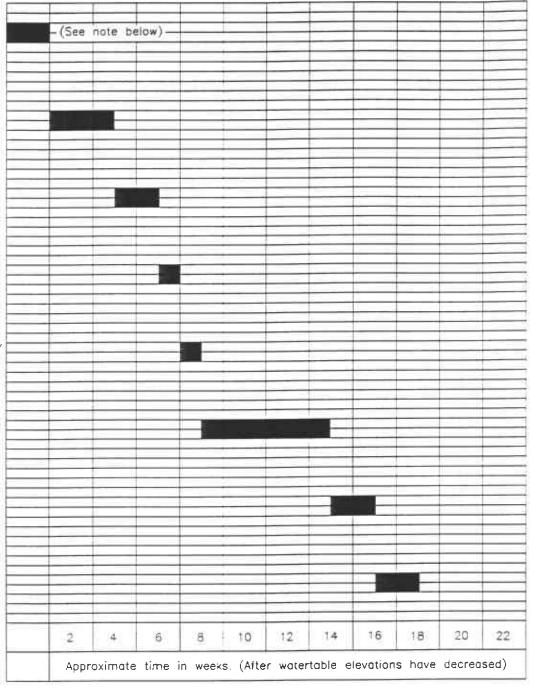
NOTE: Monthly groundwater monitoring of onsite monitoring wells will continue indefinitely until water levels decreased sufficiently (to 50 feet below grade surface) to allow for installation of air sparge well, and performance of an air sparge test.
