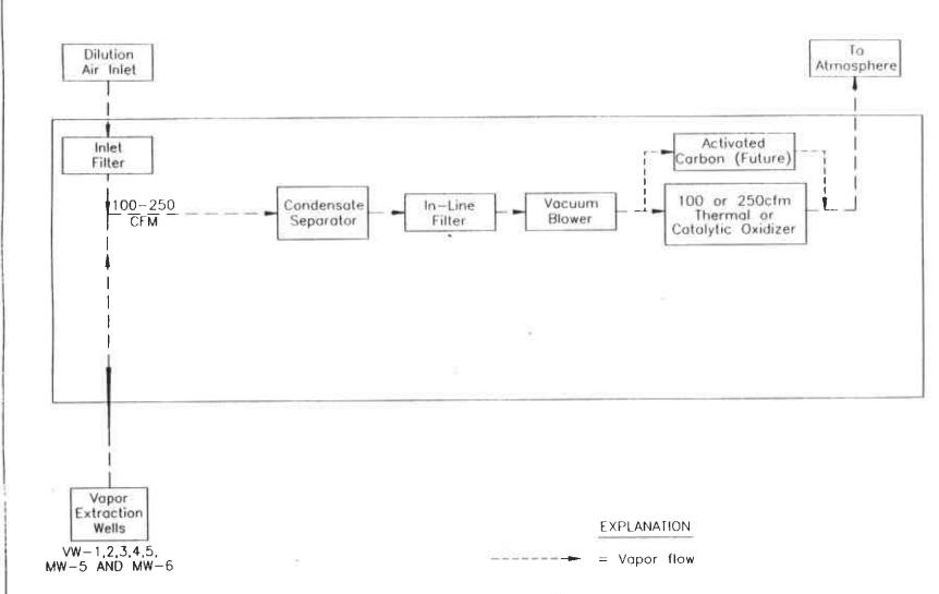
NOTE: Future Activated Carbon System may consist of two or three 1,200 lb carbon canister in series
