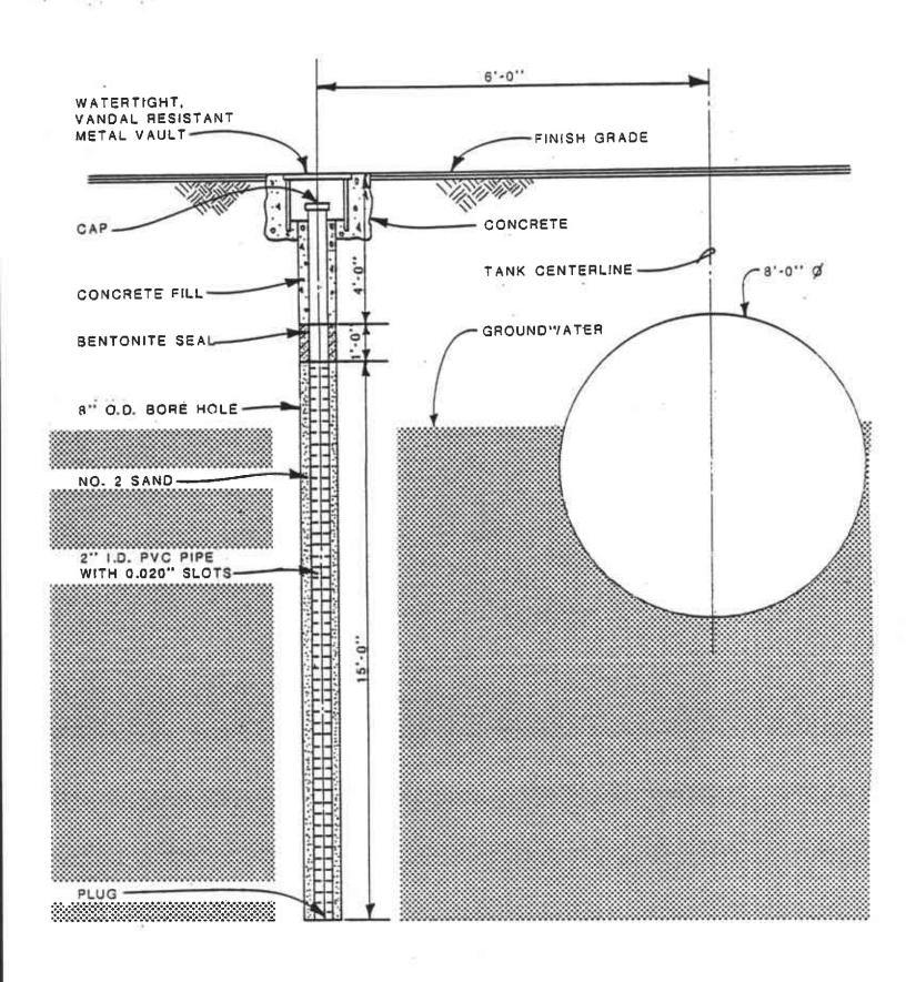
Figure 2. MONITORING WELL CONSTRUCTION
