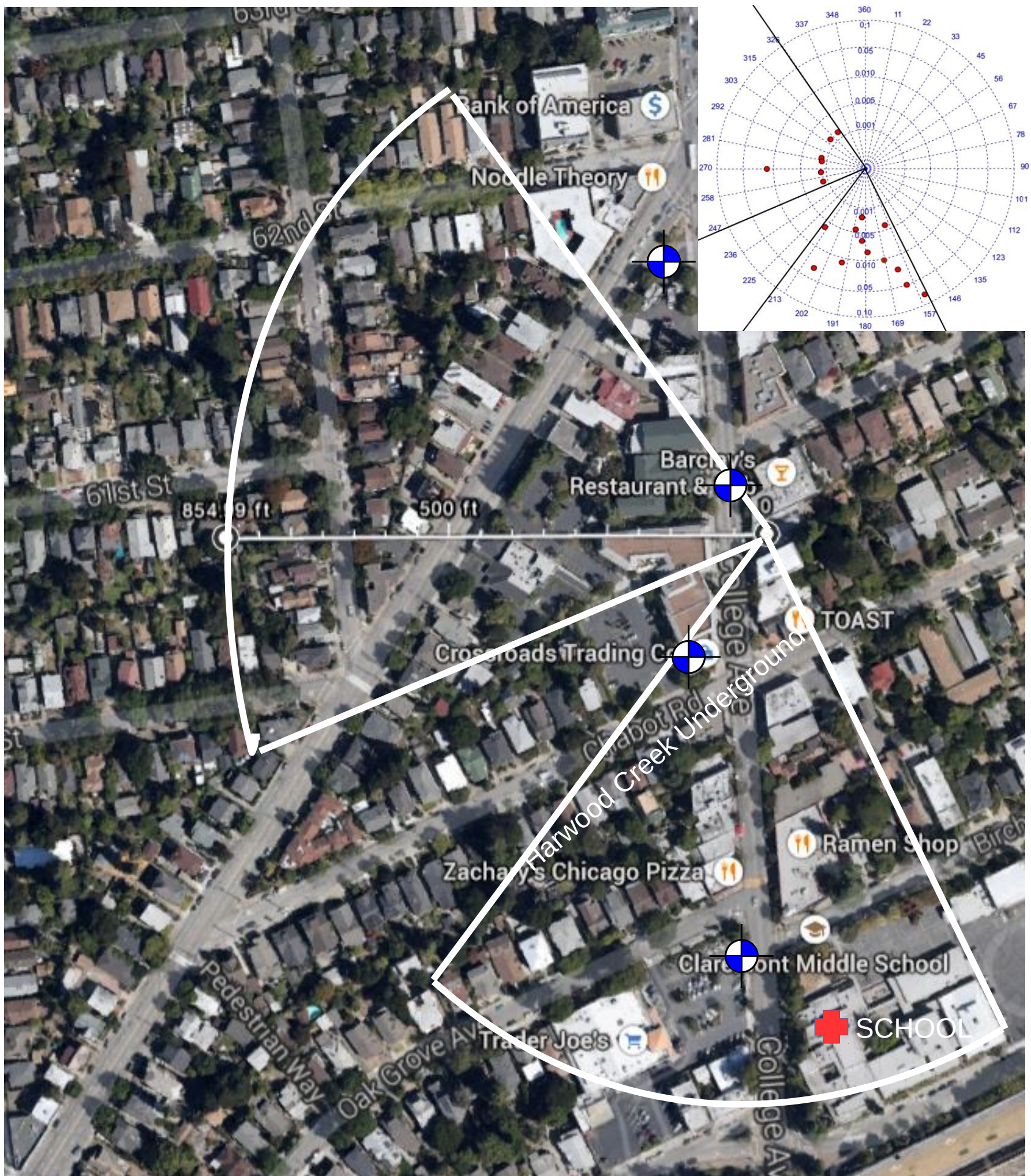
Sensitive receptor survey showing plume map for Total Petroleum Hydrocarbons (TPH) as gasoline with radius of 855 feet in two groundwater flow directions as determined from rose diagram of historical groundwater measurements.
