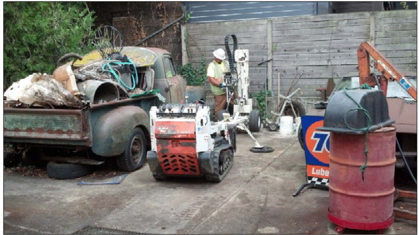
Photograph No. 4 – Southeast view of rear concrete-paved storage yard, showing EnProbe representative during drilling/ soil sampling of Boring B28 in vicinity of rear yard of adjacent residential property (GGTR, Nov. 2015).
