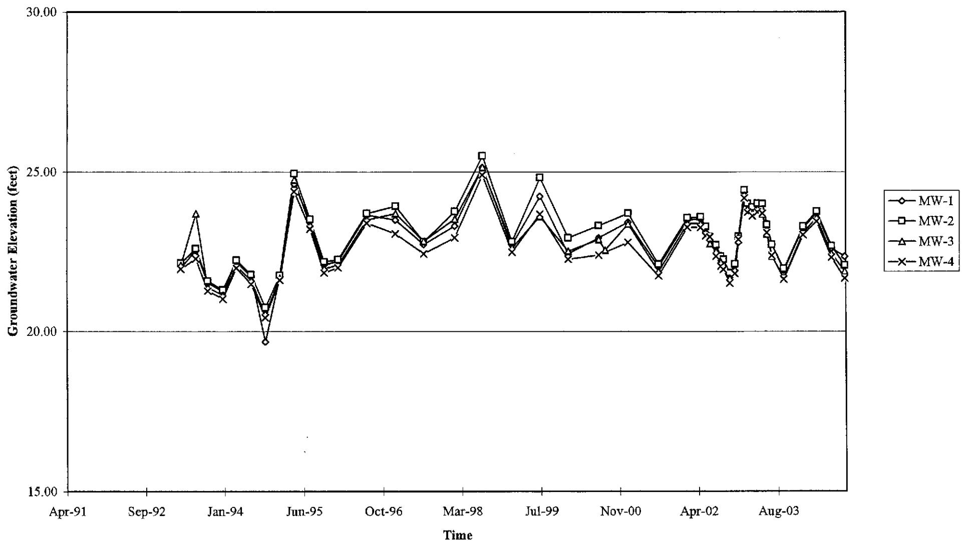
Groundwater Elevations vs. Time
