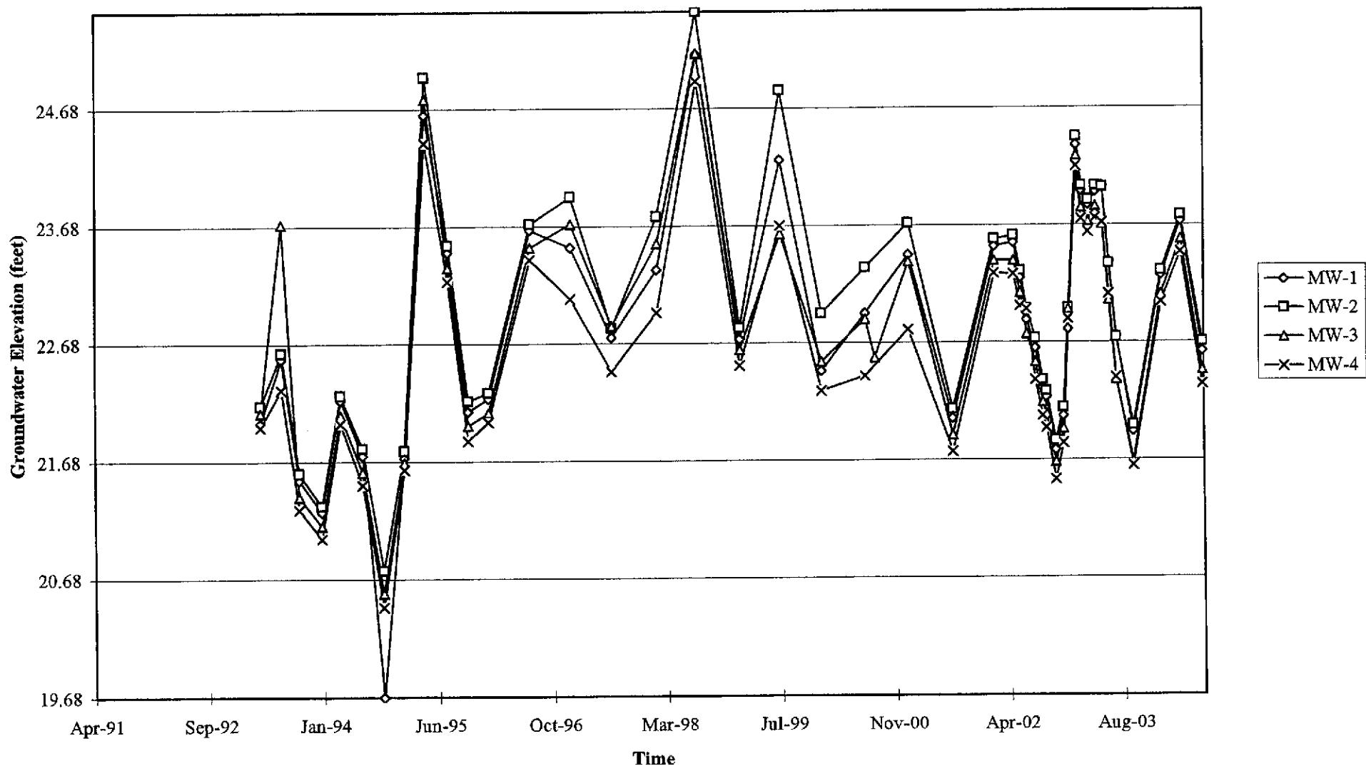
Groundwater Elevations vs. Time
