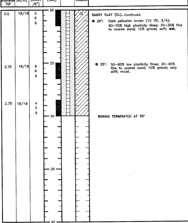
Boring was drilled using eight-inch outside diameter (OD) hollow-stem augers. Soil samples were collected using a two-inch OD split-spoon sampler at five foot intervals. A groundwater monito-ring well was installed using two-inch diameter PVC easing (see attached well detail). RG#46.03; Exp.
