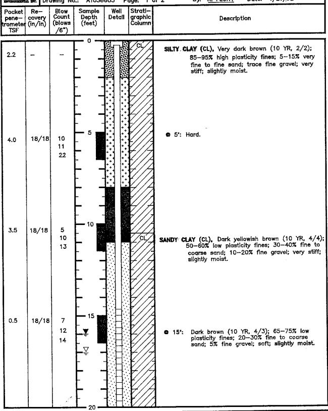
NOTES: Boring was drilled using eight—inch outside diameter (OD) hollow—stern augers. Soil samples were collected using a two—inch OD split—spoon sampler at five foot intervals. A groundwater monito—ring well was installed using two—inch diameter PVC casing (see attached well detail).
