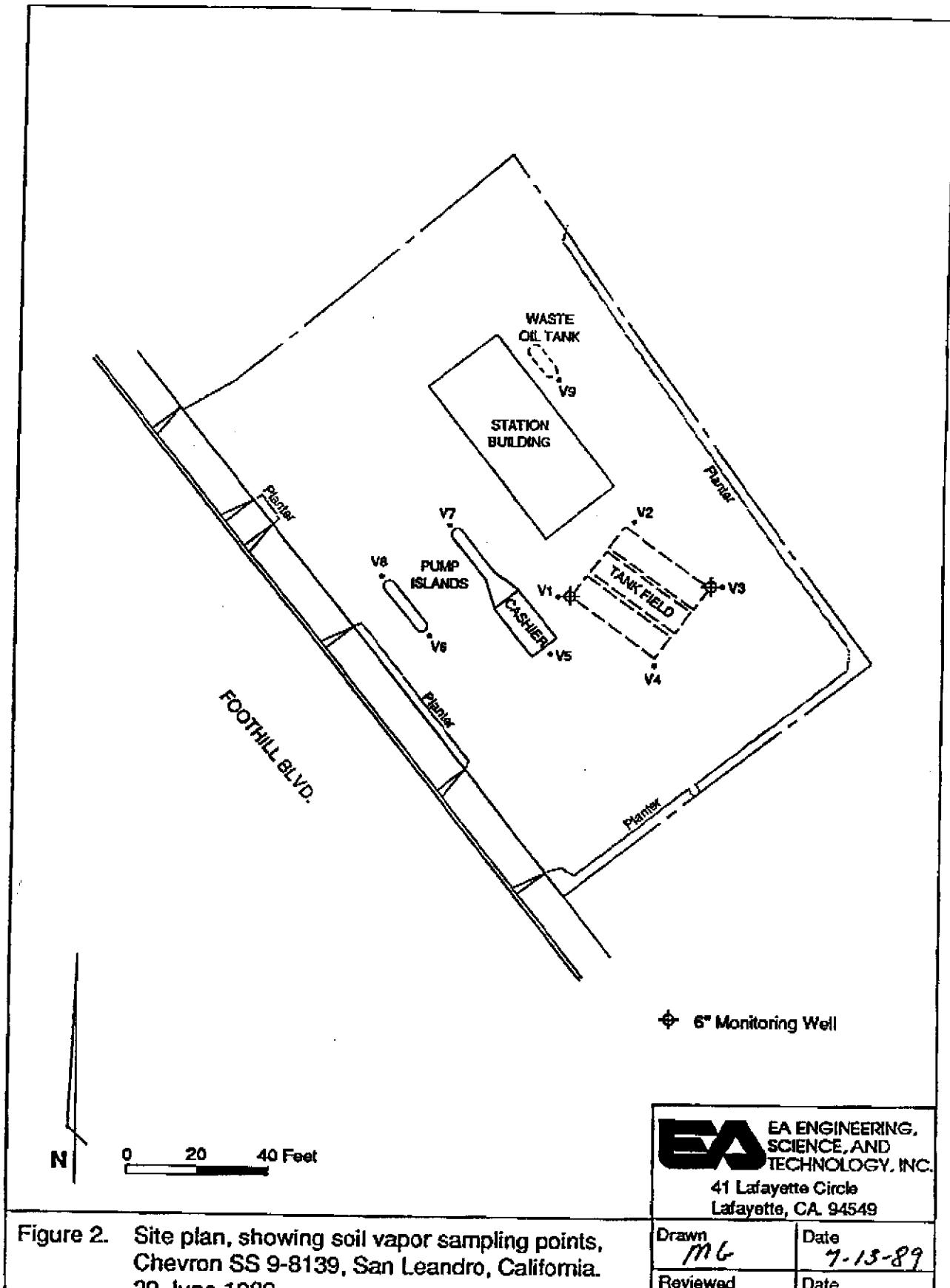
Figure 2. Site plan, showing soil vapor sampling points, Chevron SS 9-8139, San Leandro, California. 29 June 1989.
