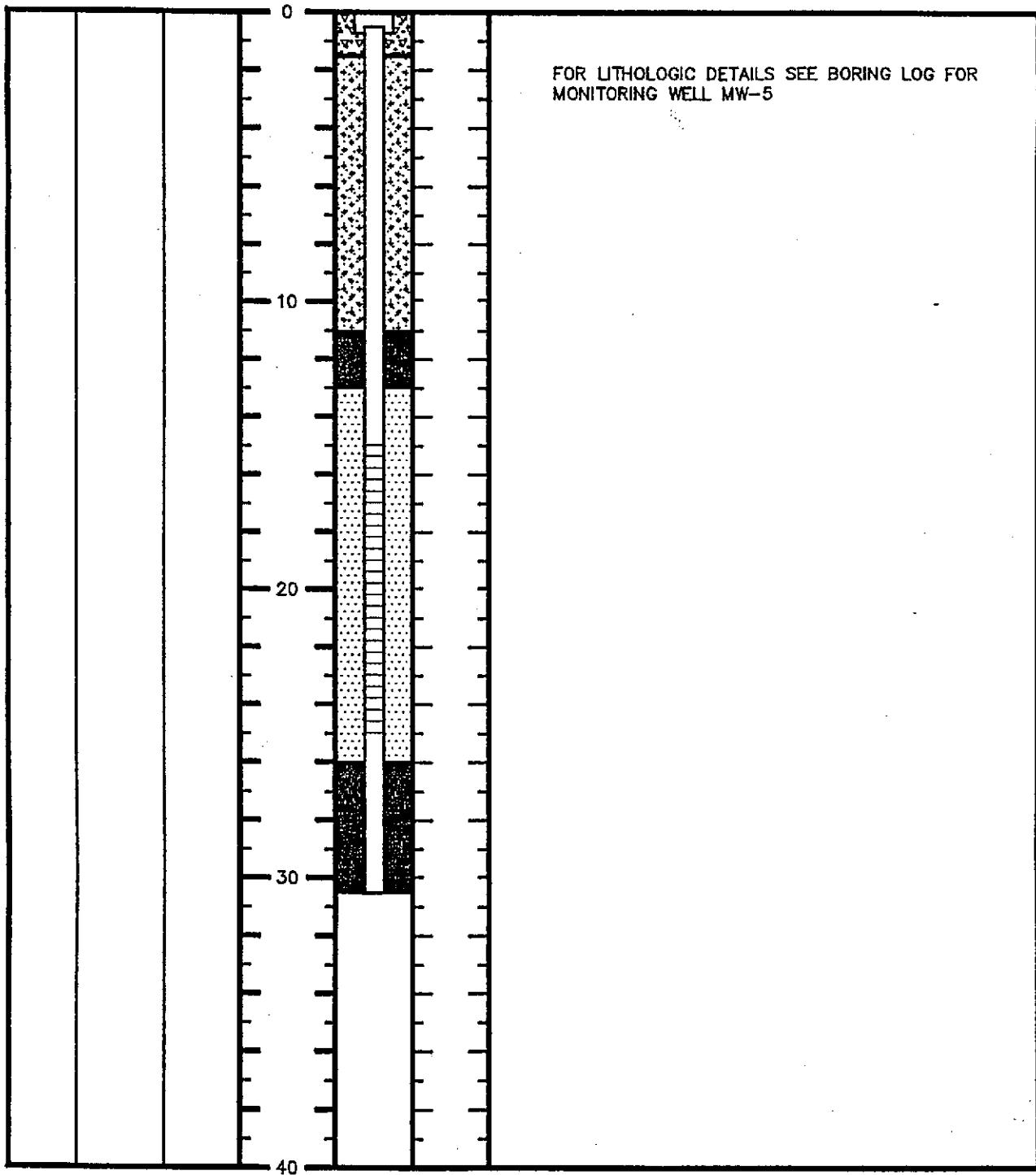
NOTES: Monitoring well Mw-5 was decommissioned with 8" diameter hollow-stem augers to 30ft. Boring was reamed with 10" diameter hollow-stem augers to 30.5ft. A groundwater extraction well was installed using 4" diameter sch 40 PVC and 0.010" machine slotted PVC screen.
