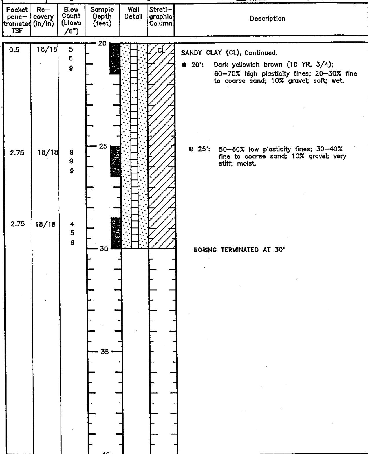
NOTES: Boring was drilled using eight-inch outside diameter (OD) hollow-stem augers. Soil samples were collected using a two-inch OD split-spoon sampler at five foot intervals. A groundwater monitoring well was installed using two-inch diameter PVC casing (see attached well detail).
