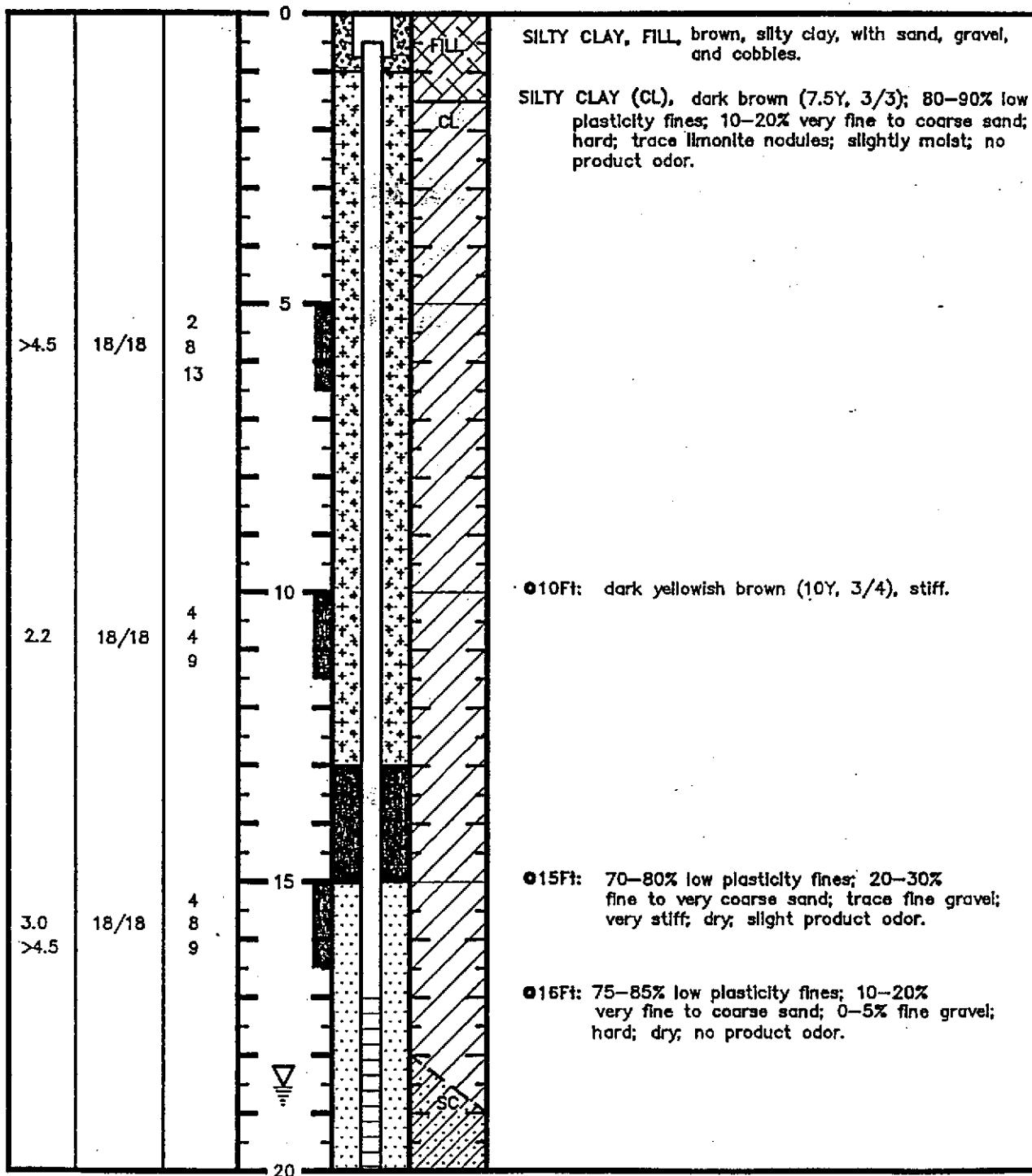
NOTES: Boring was drilled with 8" outside diameter hollow-stem augers. Soil samples were collected at 5ft intervals using a 2" diameter modified-California split-spoon sampler with brass liners. A groundwater monitoring well was installed using 2" diameter sch 40 PVC and 0.010" machine slotted PVC screen.
