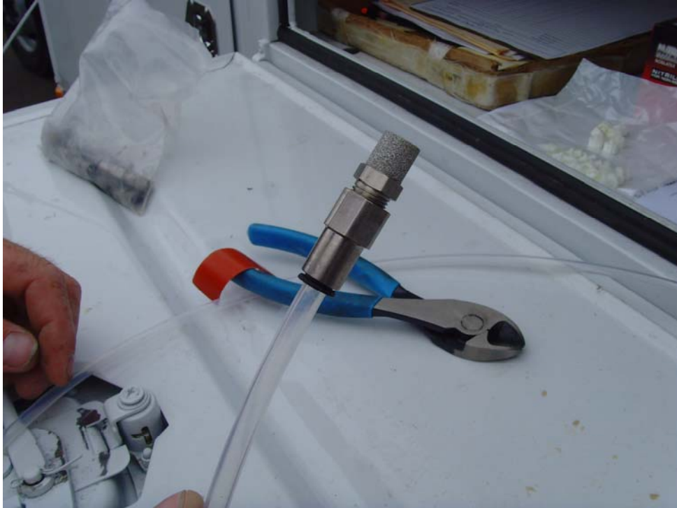
View of soil gas intake port connected to 1/4" O.D. Polytube
