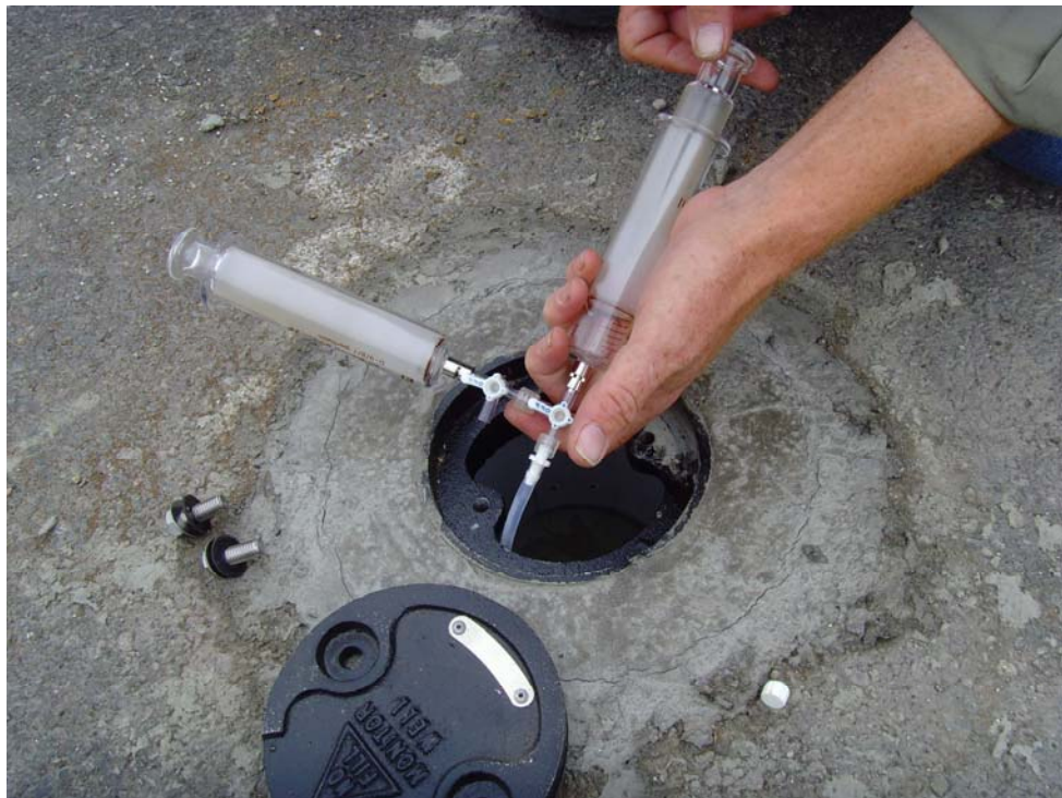
View of soil gas probe duplicate sampling
