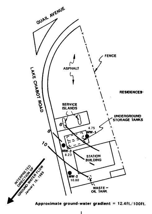
= Line of equal depth in feet to ground water
