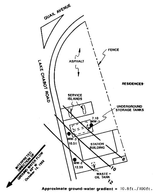
= Line of equal depth in feet to ground water
