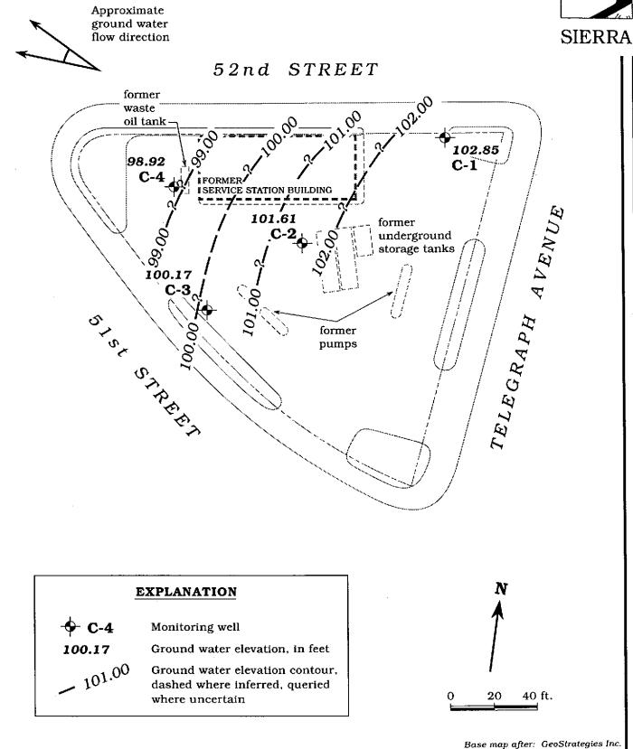
Figure 2. Monitoring Well Location and Ground Water Contour Map - September 13, 1993 - Former Chevron Service Station #9-3864, 5101 Telegraph Avenue, Oakland, California
