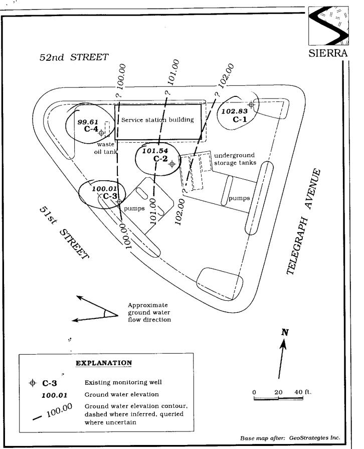
Figure 2. Monitoring Well Location Map and Ground Water Elevation Contours - June 6, 1991 - Chevron Service Station #9-3864, 5101 Telegraph Avenue, Oakland, California
