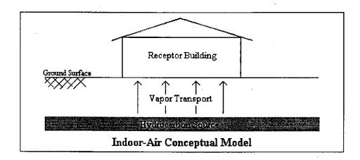
As indicated by the conceptual model, subsurface vapors transport upward into the receptor building and accumulate to a steady state concentration based on the indoor air exchange rate and building size. The formula for calculating the indoor air concentration is:
