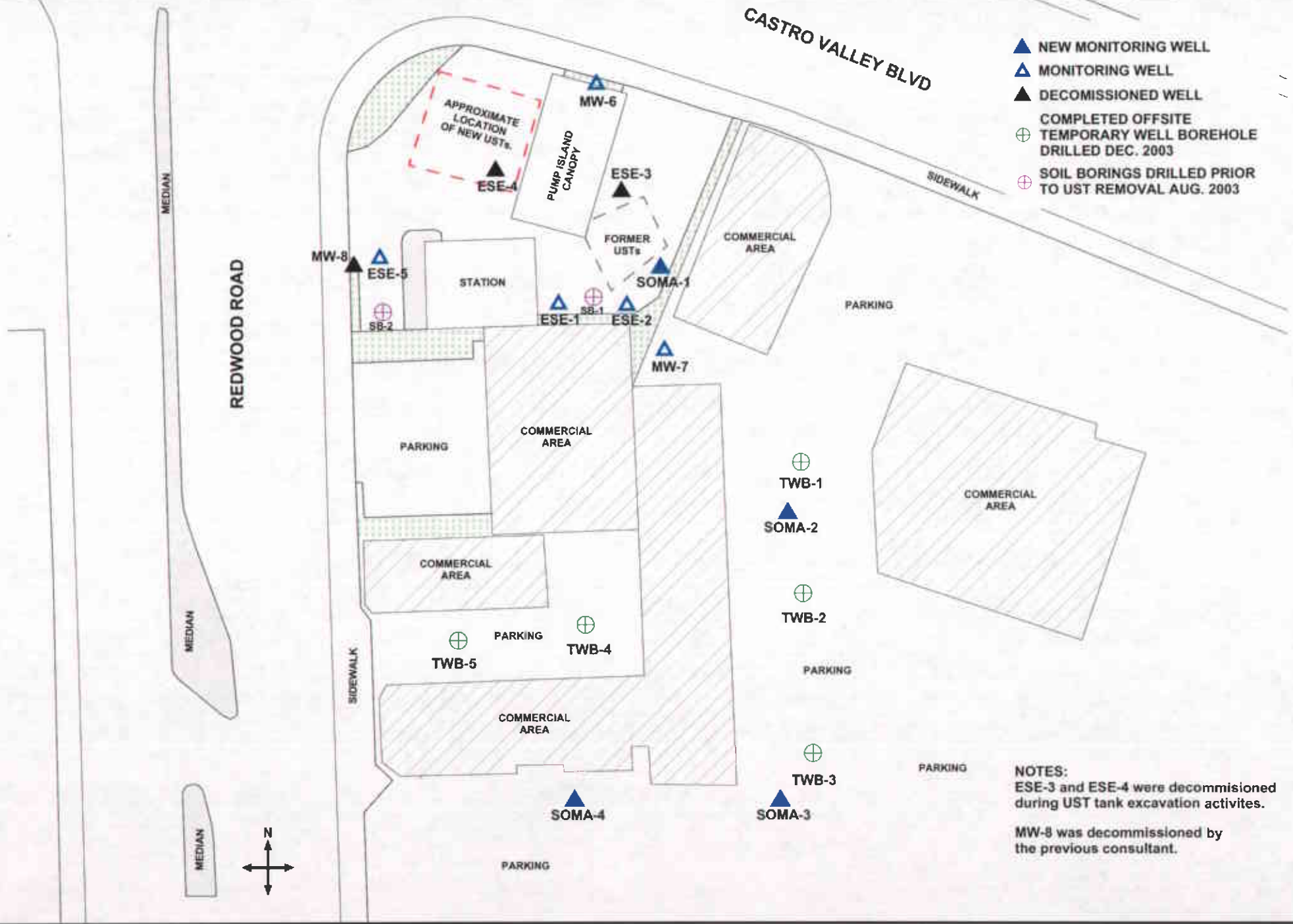
Figure 2: Site map showing locations of existing monitoring wells, decommissioned wells, offsite temporary well boreholes, and monitoring wells installed by SOMA.
