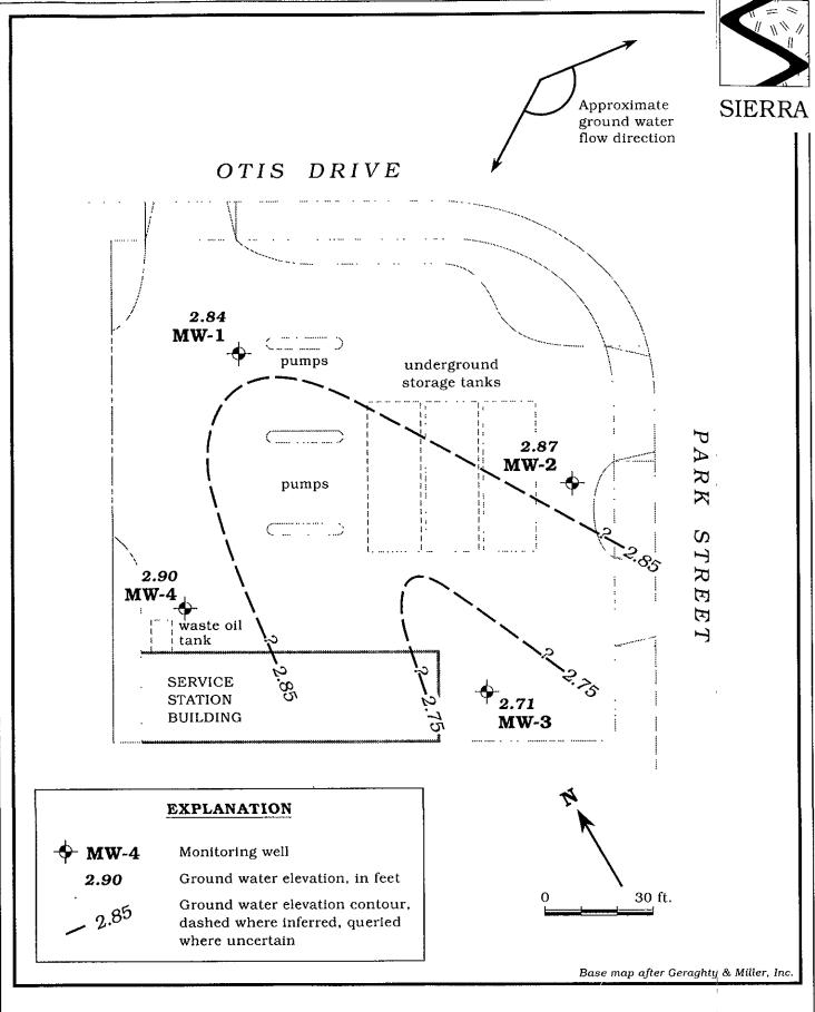
Figure 1. Monitoring Well Location and Ground Water Elevation Contour Map - October 26, 1993 - Chevron Service Station #9-6607, 2340 Otis Drive, Alameda, California
