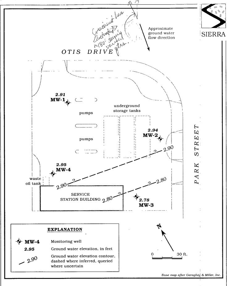
Figure 1. Monitoring Well Location and Ground Water Elevation Contour Map - July 14, 1993 - Chevron Service Station #9-6607, 2340 Otis Drive, Alameda, California
