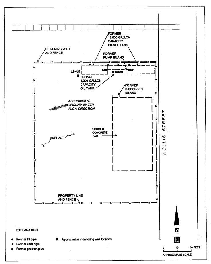
Figure 2: SITE PLAN SHOWING MONITORING WELL LF-31
