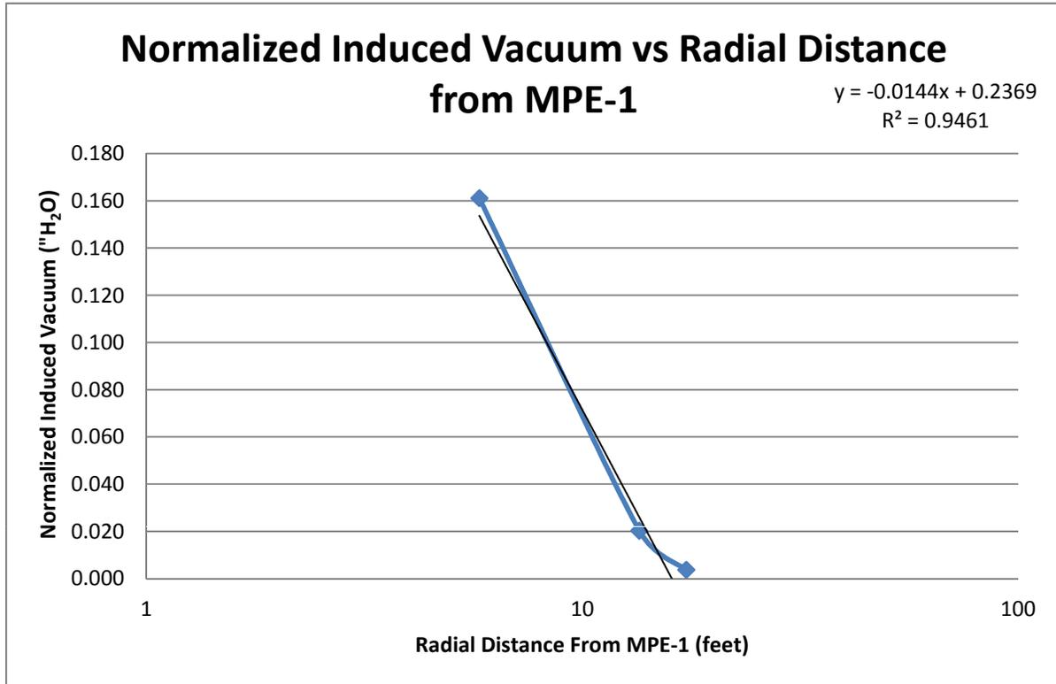
Resulting linear equation for normalized induced vacuum:
