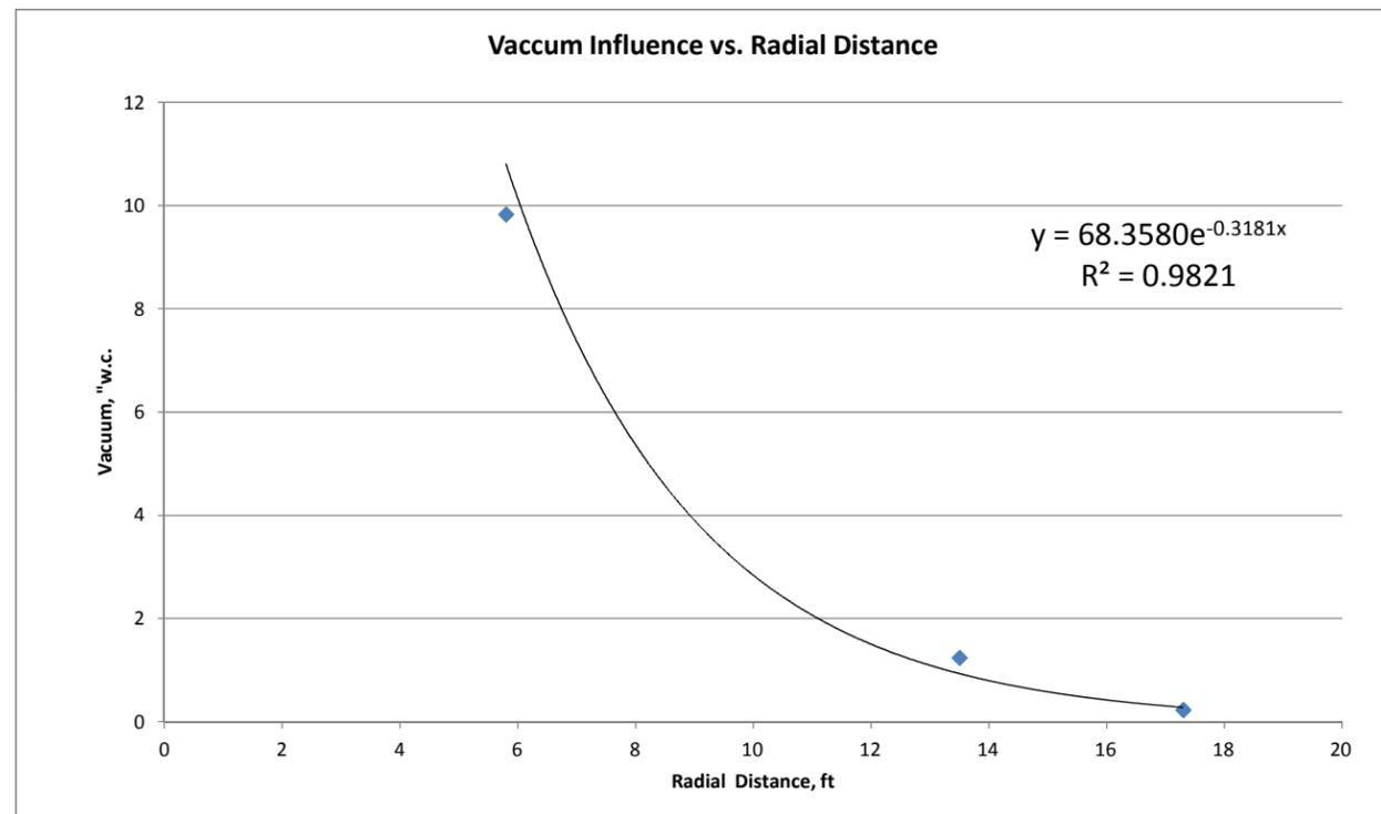
**SVE Pilot Test ROI Calculation - Pore Volume Exchange Rate**
