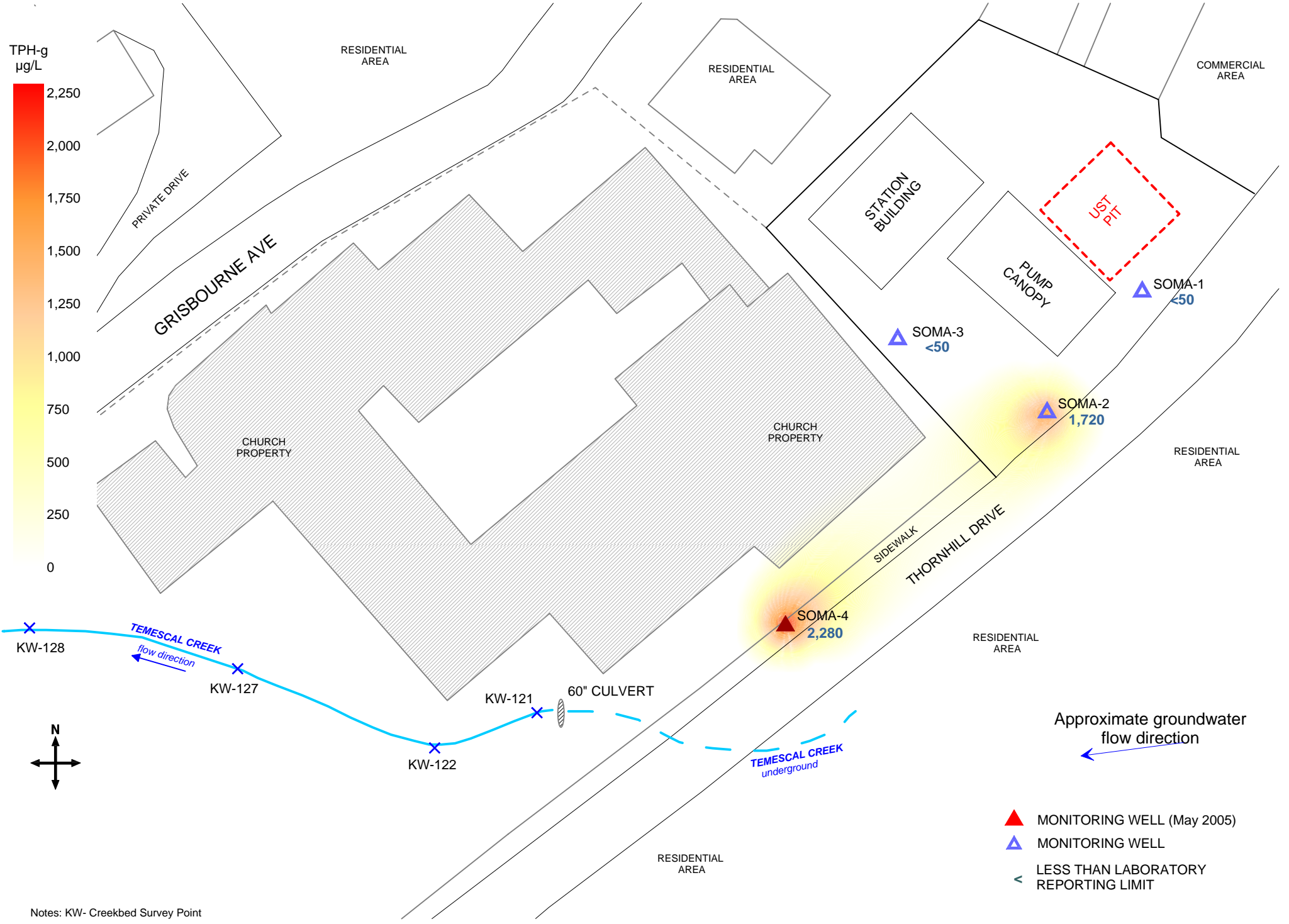
Figure 4: Contour map of TPH-g concentrations in groundwater. January 8, 2007.
