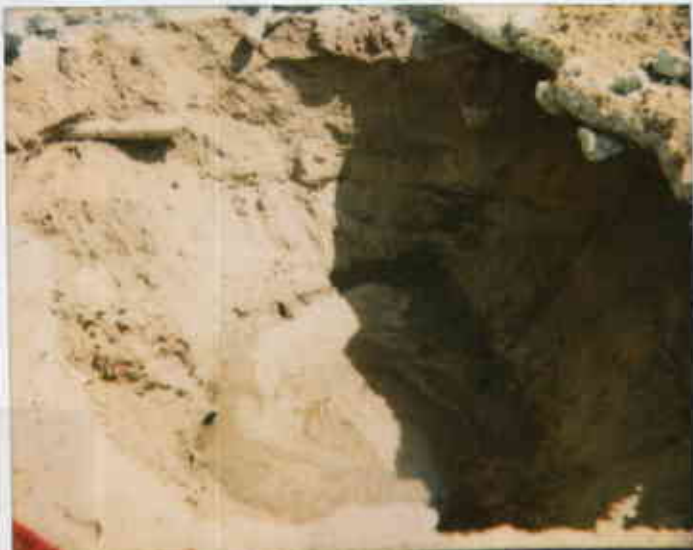
North pit appears clean, i.e. no staining
