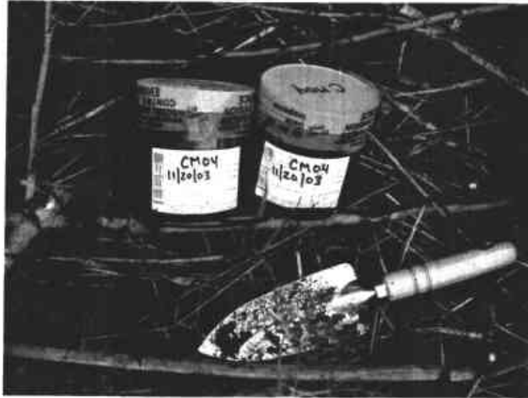
Photo no. 15: Sample CM04 after it was taken from inside of tank T-1.
