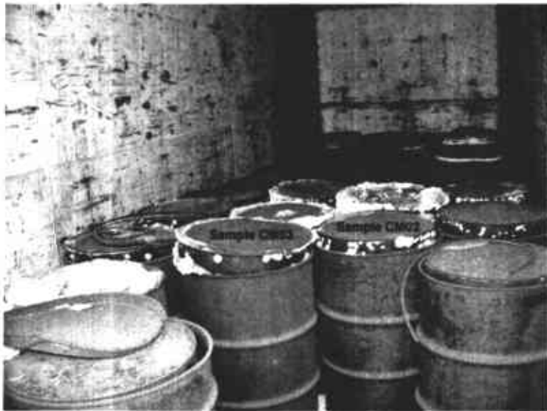
Photo no. 7: Thirty-six 55-gallon drum containing caustic solids inside of trailer no. 4. Samples CM02 and CM03 were taken from the labeled drums.
