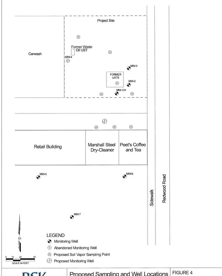
BSK Associates Engineers Laboratories Proposed Sampling and Well Locations
