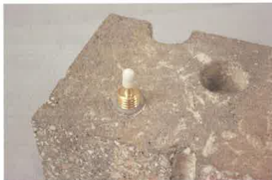
Figure 4. Installed Vapor Pin™.
