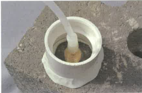
Figure 6. Water dam used for leak detection.
