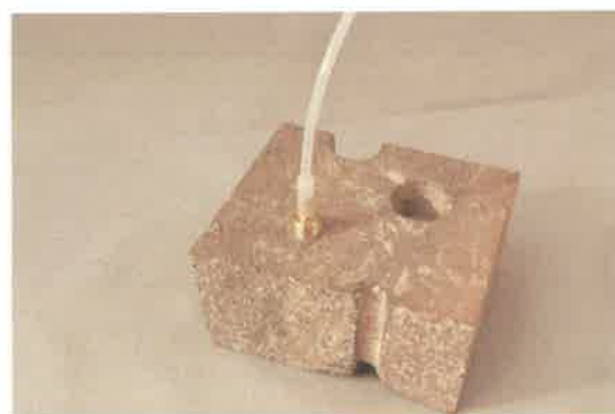
Figure 5. Vapor Pin™ sample connection.
