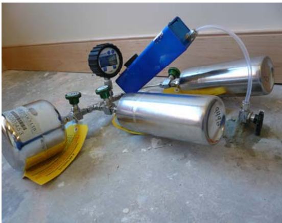
Typical sub-slab sampling manifold and encasement within Shroud with IPA atmosphere.
