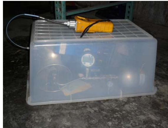
Typical sub-slab sampling manifold and encasement within Shroud with IPA atmosphere.
