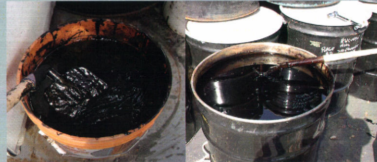
Tar-Like Material Deposited Inside Knock out Tank of Dual-Phase Extraction System
