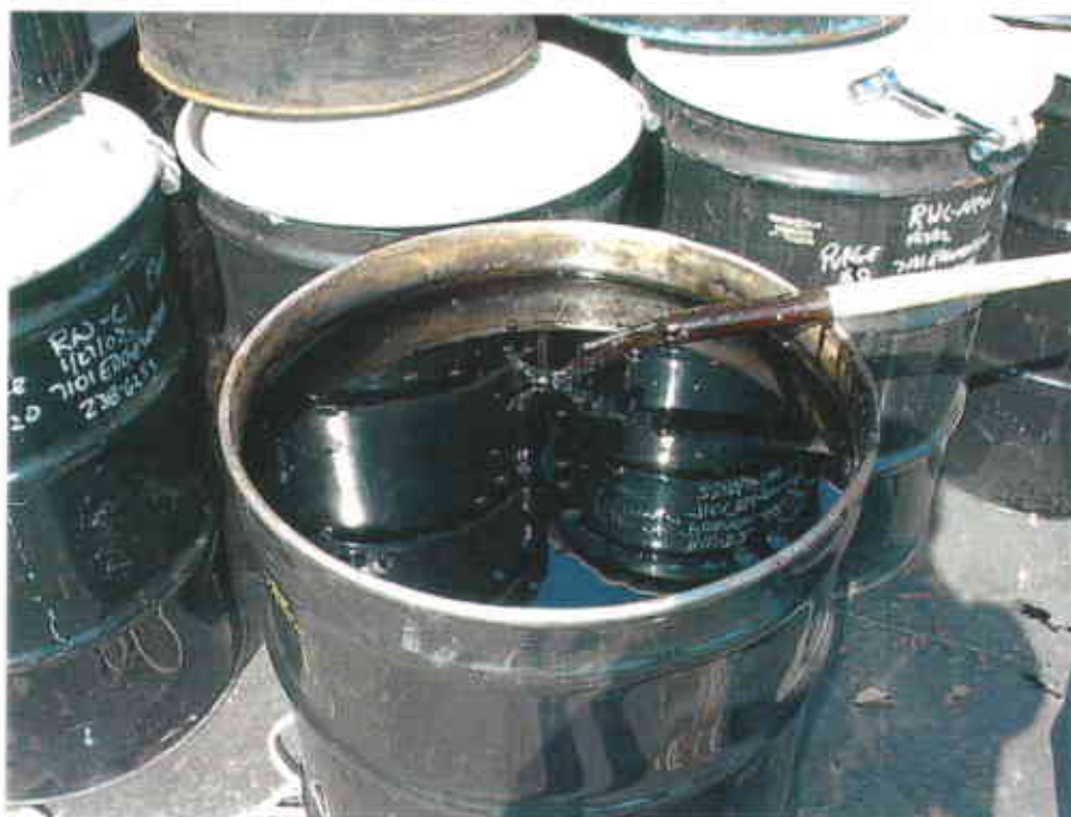
Photo 7: Separate-phase hydrocarbons recovered from extraction wells.
