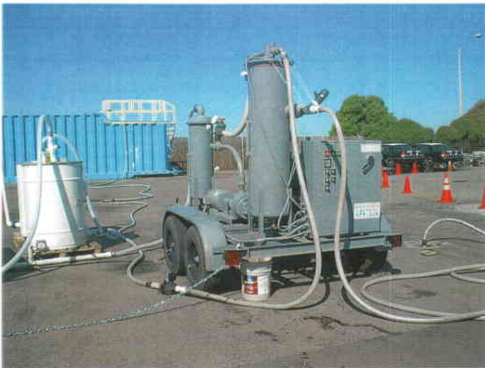
Photo 1: Trailer mounted Dual-Phase Extraction (DPE) system
