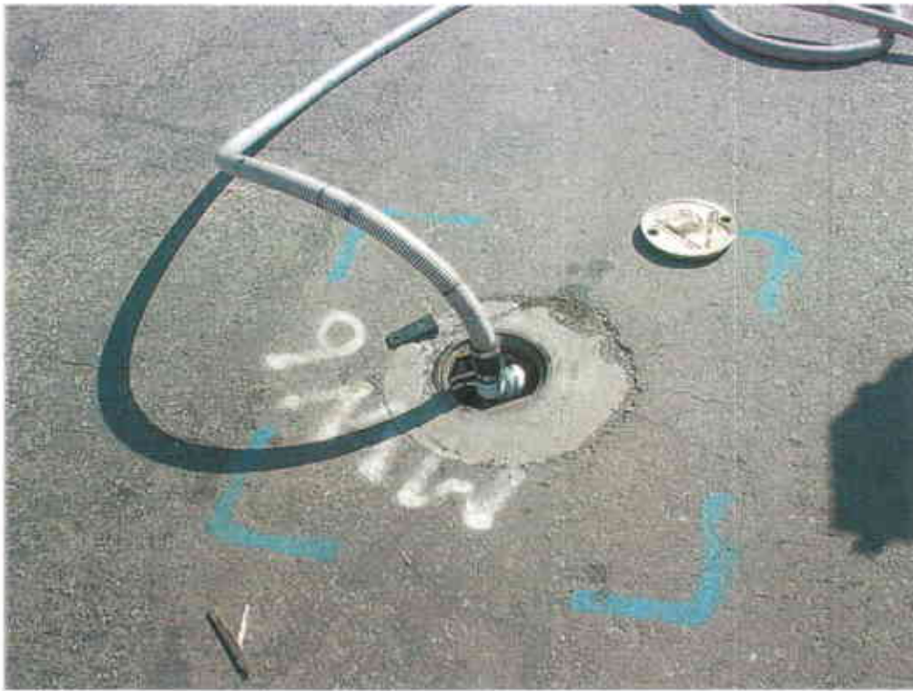
Photo 3: Dual-phase extraction from Well MW-6.
