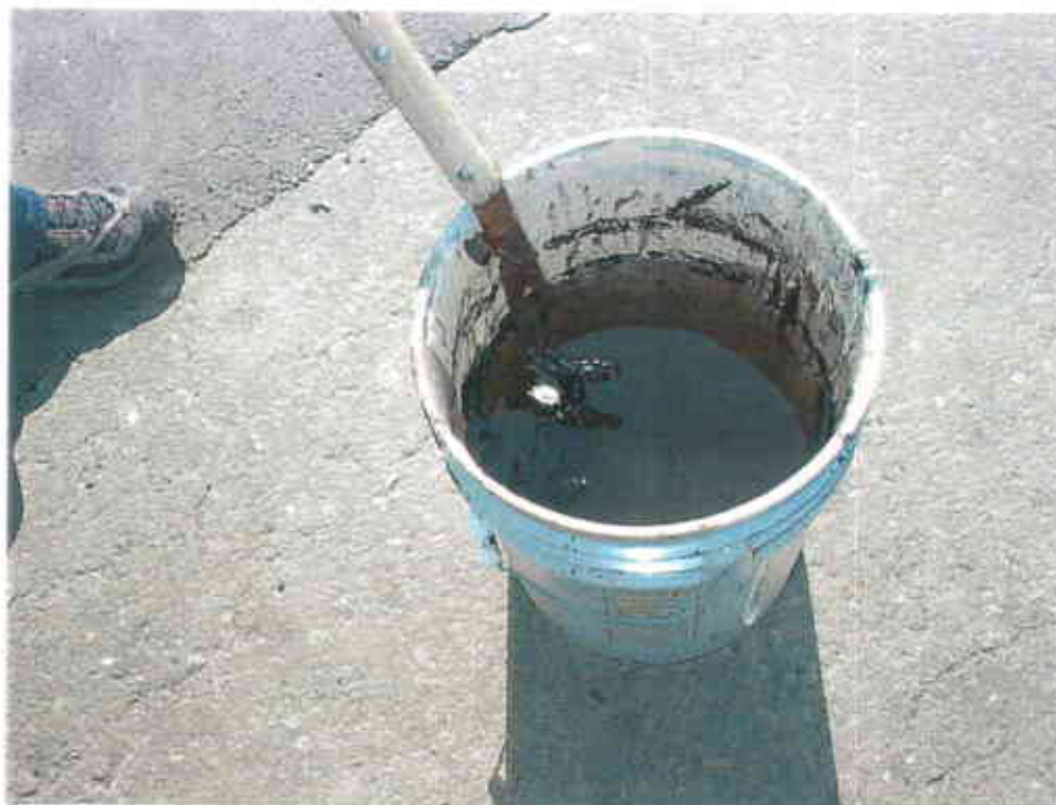
Photo 6: Tar-like material floating on surface of extracted groundwater. The material is in a semi-solid state and very sticky.
