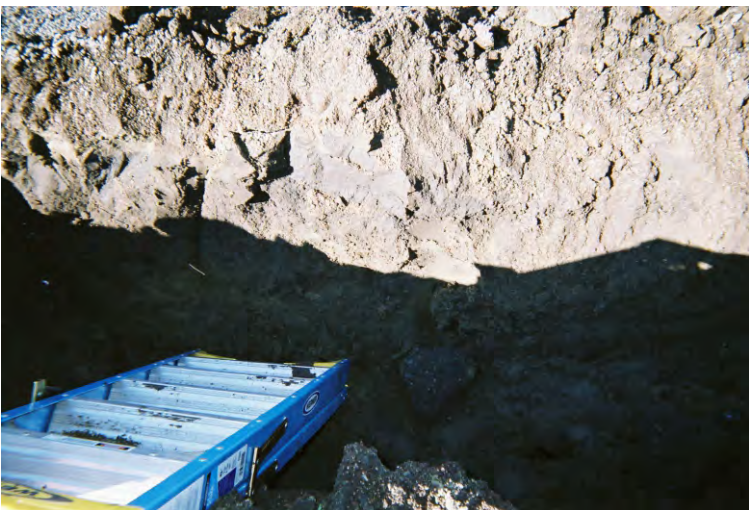
1½ to 2½ ft bgs is a natural silty clay, black, soft and moist. 2½ to >4 feet bgs is a clayey silt, light olive green, soft and moist.
