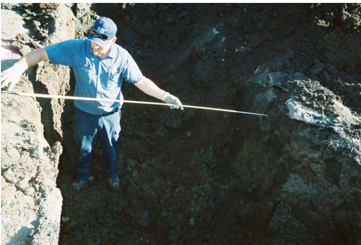
Photo 27 - Width of the original gasoline UST pit is shown to be 7 feet across, and a depth of approximately 4 feet. The olive green clayey silt was observed at the bottom of the trench.
