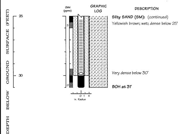
Well Construction and Boring Log - Former Chevron Service Station #94816
