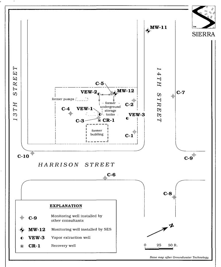
Figure 1. Monitoring, Vapor Extraction and Recovery Well Locations - Former Chevron Service Station #9-4816, 301 14th Street, Oakland, California
