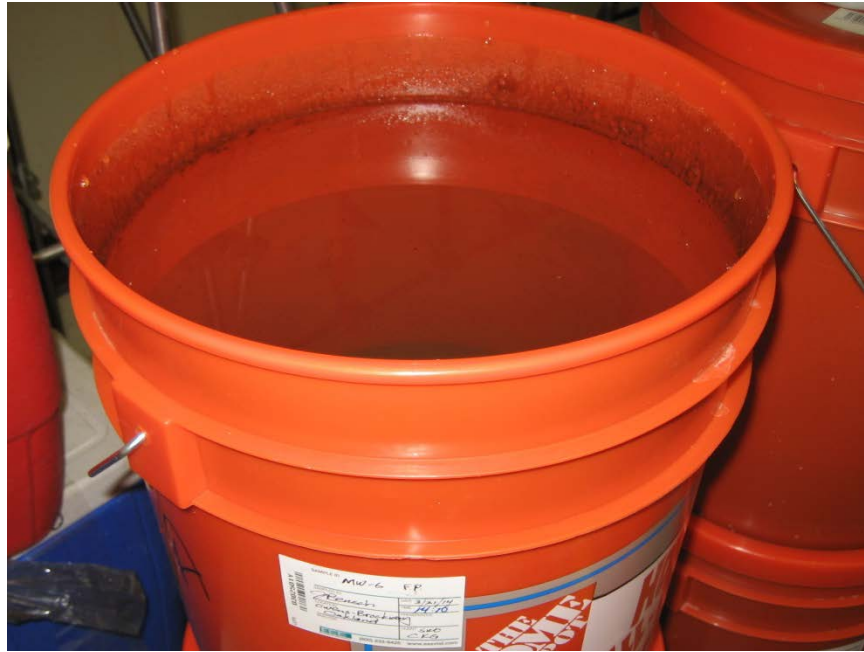
Figure 4. Example of Free Phase Residue above Waterline (MW-6).
