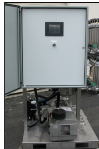
Touch-screen HMI is mounted on a swing-out door behind exterior panel door.
