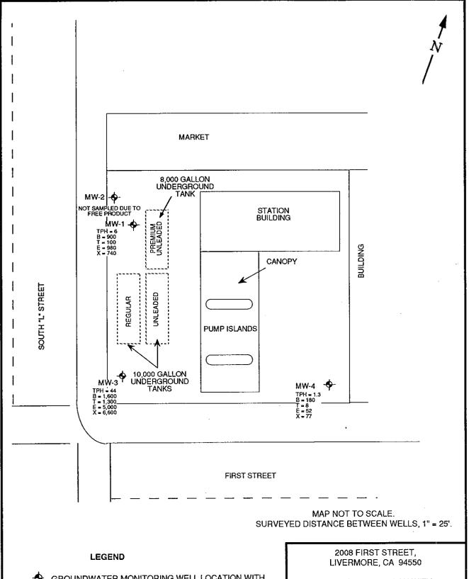
GROUNDWATER MONITORING WELL LOCATION WITH TPH CONCENTRATIONS IN mg/L and BTEX CONCENTRATIONS IN µg/L
