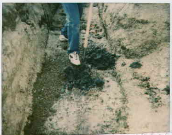
7225 Bancroft Ave, Oakland 8/27/96 Juliet S. 05617107379-24 1438 9351 COPIES & ENLARGEMENTS CALL 800-421-1030 Sample collected from piping trench adjacent to middle dispenser had strong odor in fill above clay. Fives moisture & broken water lines.
