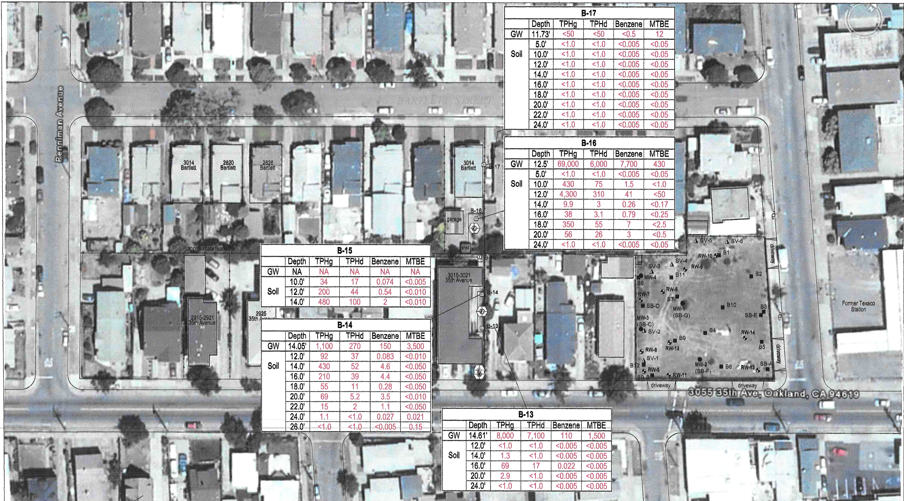
FIGURE 5 AF OFFSITE PHASE I HYDROCARBON CONCENTRATIONS in SOIL and GROUNDWATER with PROPOSED SOIL BORING LOCATIONS FORMER EXXON STATION 3055 35th AVENUE Oakland, California
