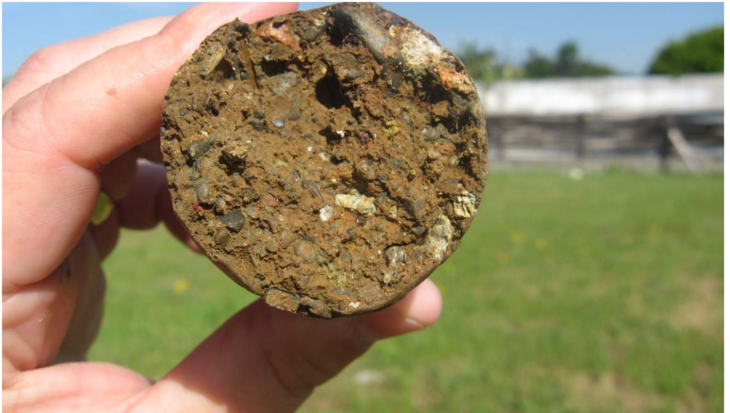
003.Lower permeability Gravelly Lean Clay encountered in all borings below 17-20 feet bgs
