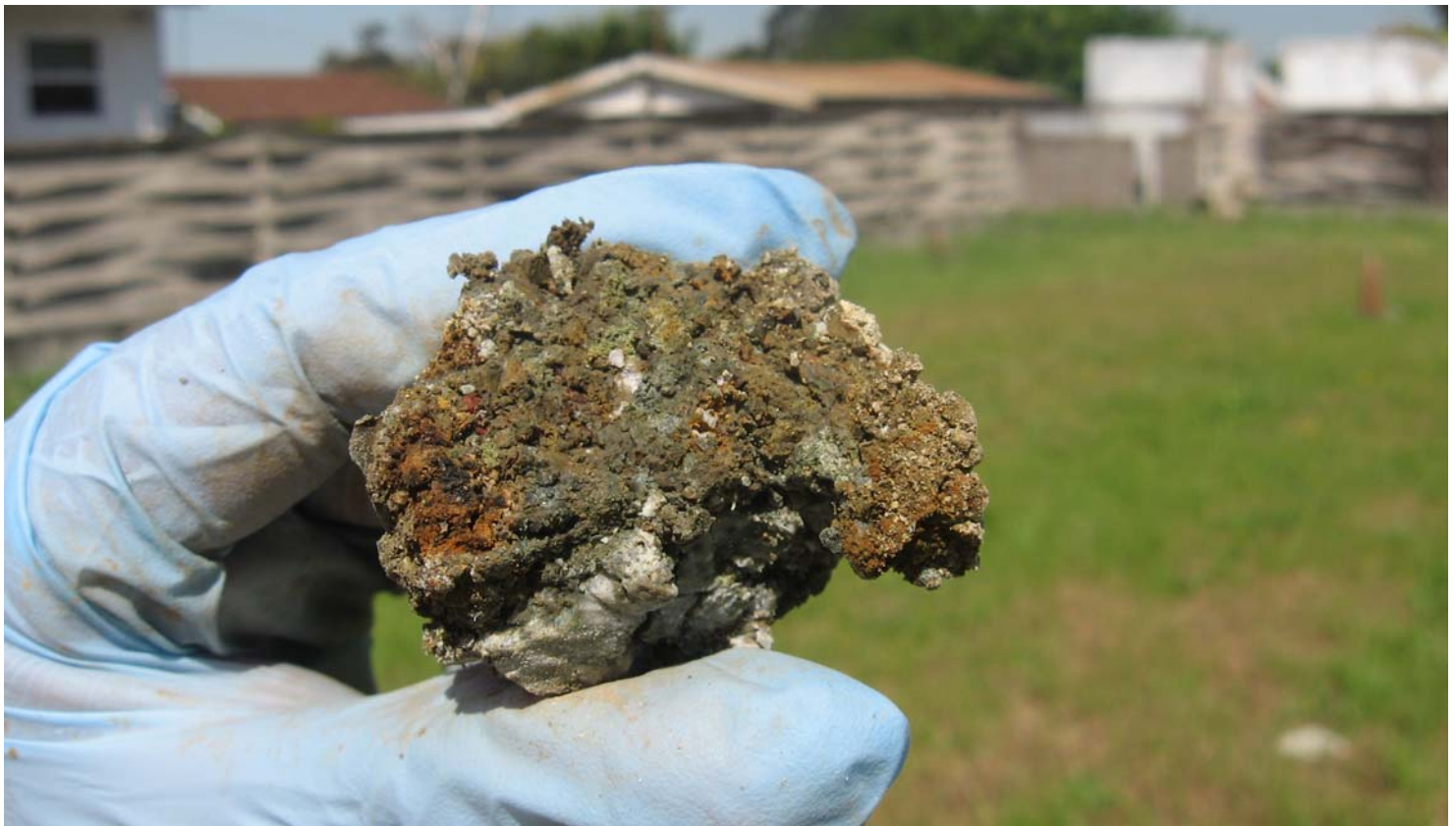
002. Subsurface lithology dominantly comprised of lower permeability Clay-Sand-Gravel mixtures
