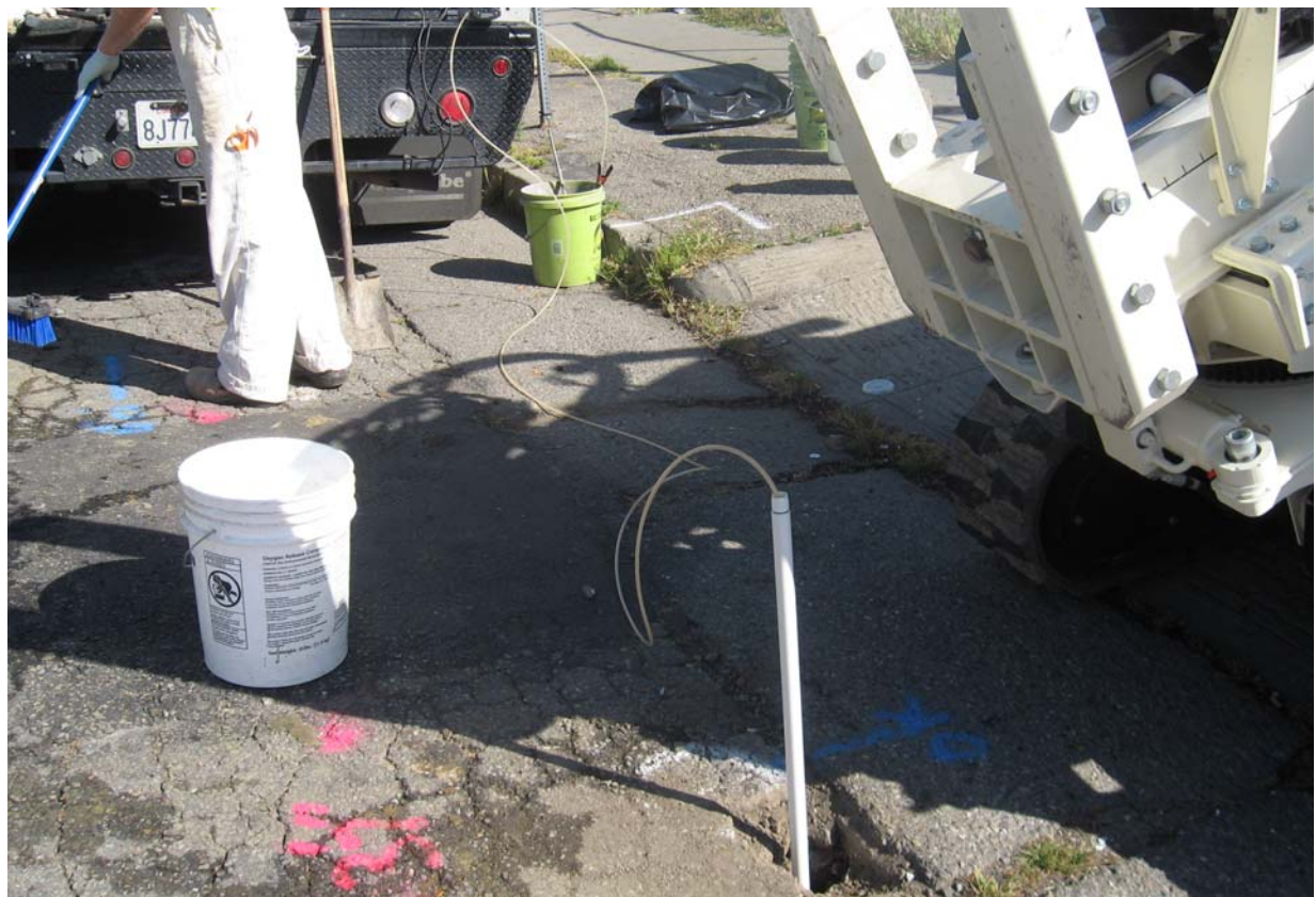
015. Collecting grab groundwater sample from boring DP-2
