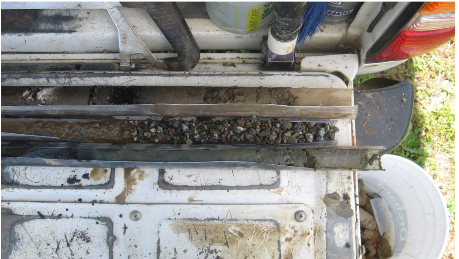
005.Saturated tank pit fill materials
