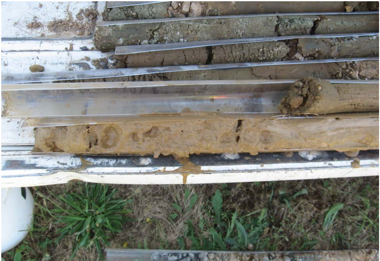
012.Narrow, confined saturated zone encountered from 29-30 feet bgs in DP-3
