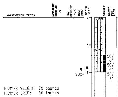
EQUIPMENT 3" Solid Flight Auger DATE DRILLED 9/17/90
