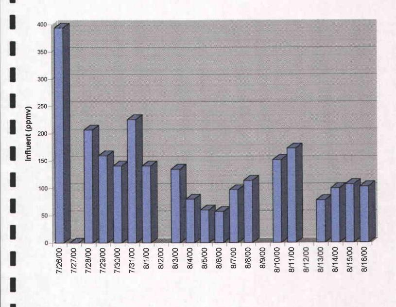
Figure 5: Influent Organic Carbon Concentrations, as Measured with PID
