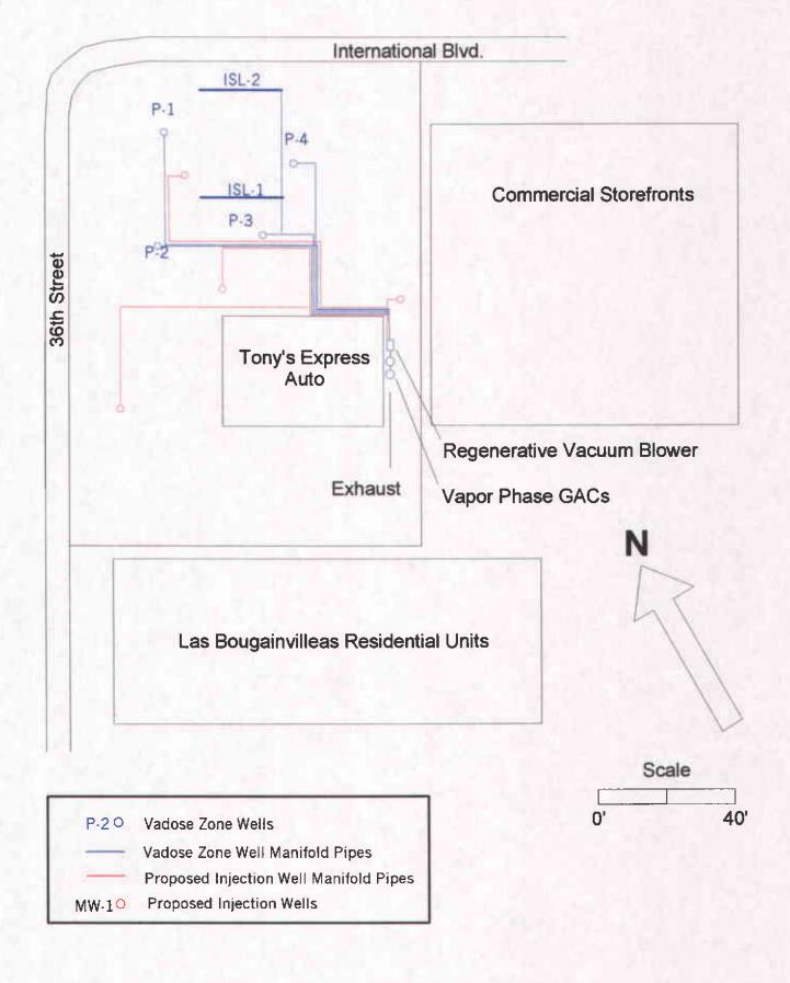
Figure 2: Location of Vapor Extraction Wells
