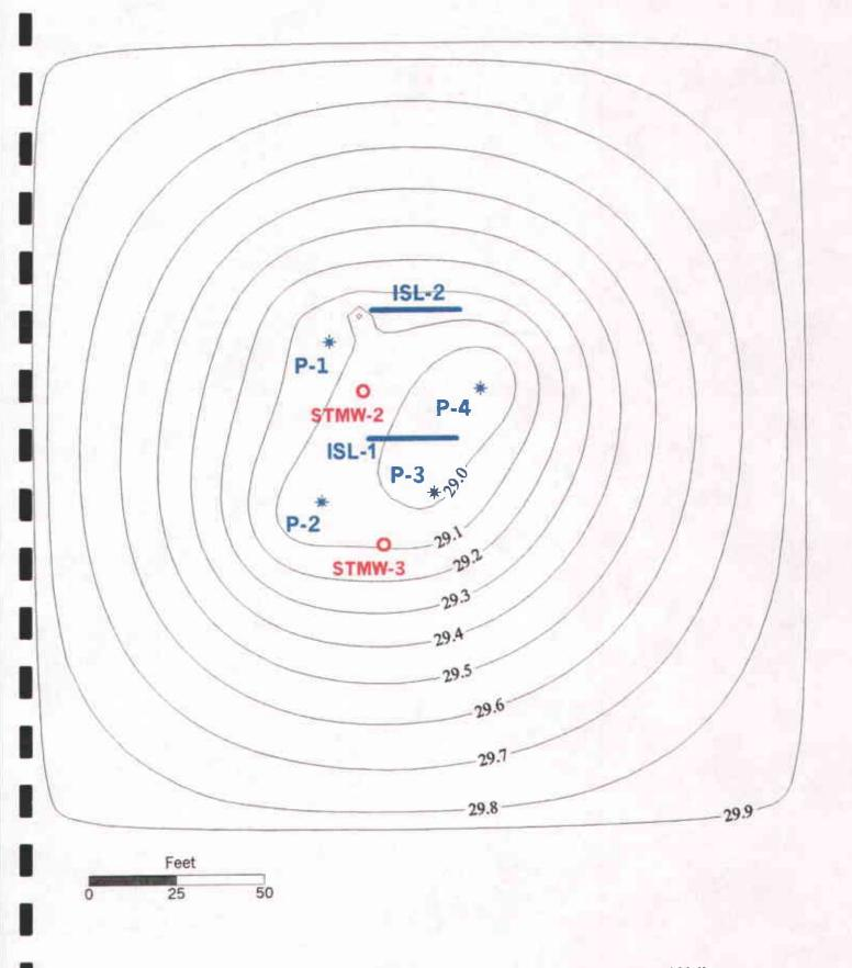
Figure 4: Simulated Pressure Contours around Vapor Extraction Wells
