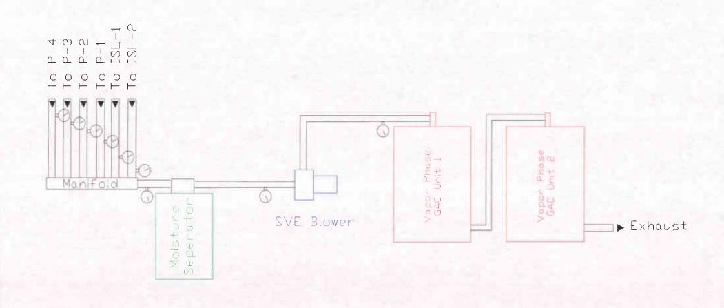
Figure 3: Schematic of the Vapor Extraction System
